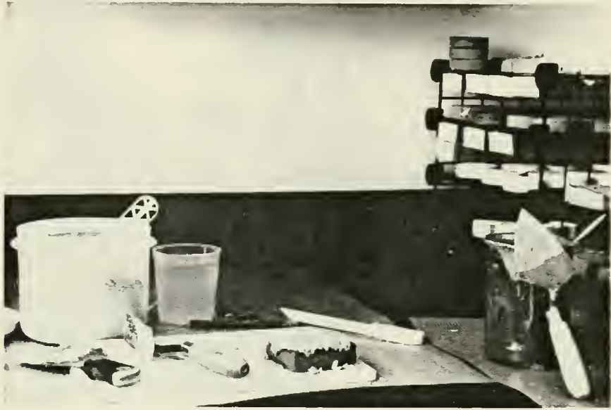
Lime plaster application on adobe blocks, first coat.
