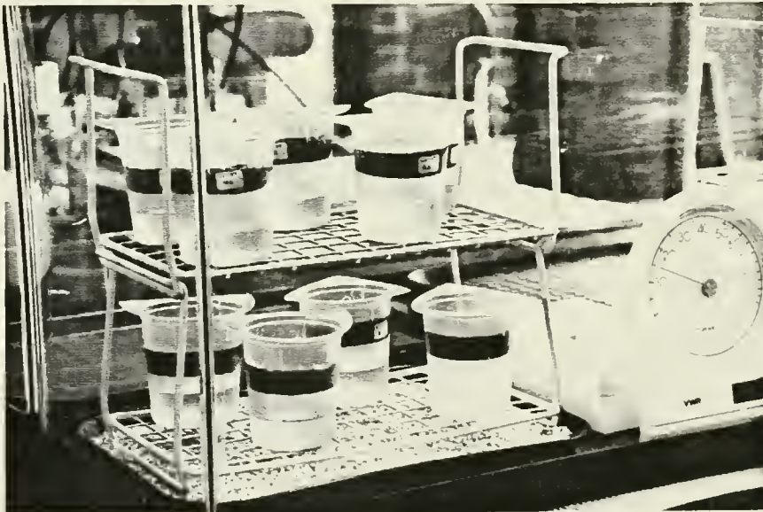
Dish assemblies with clay plaster samples on dry chamber, at 15% Relative Humidity.
