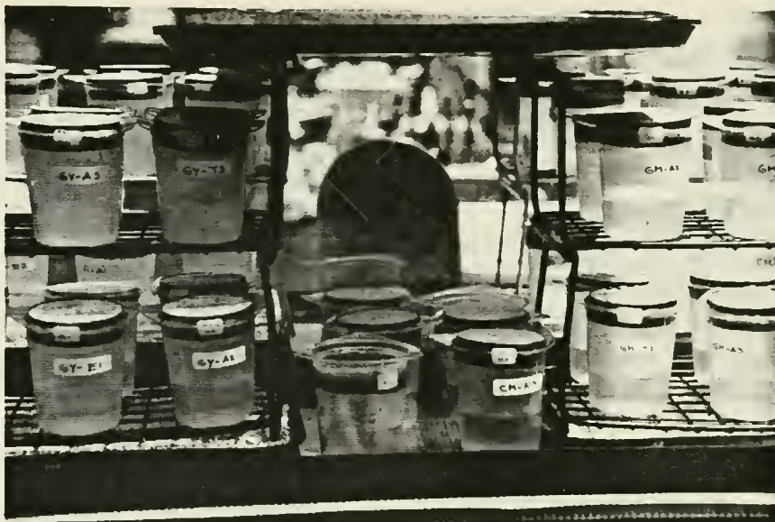
Dry chamber with Gypsum, Clay/lime and Gypsum/lime samples
