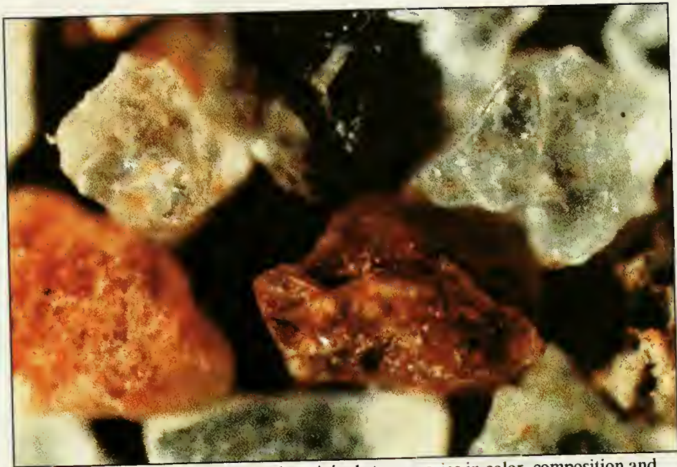
Figure 6.6. Aggregate used for the original stucco varies in color, composition and particulate shape. As shown, aggregate removed from matrix by digestion with hydrochloric acid. Reflected light @ 40x magnification.
