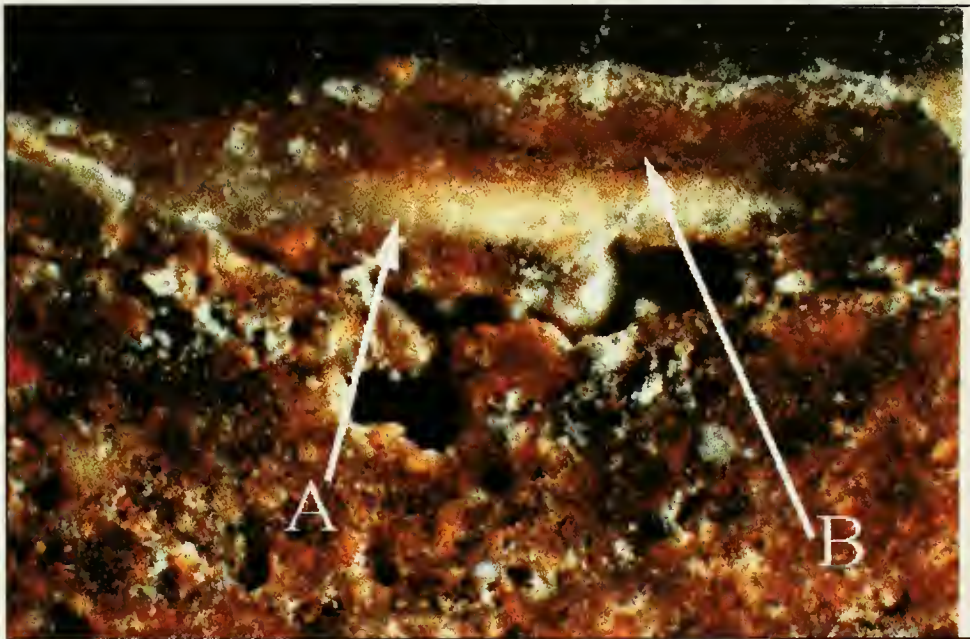
Figure 6.4 Aiken-Rhett Sample 101.2, first floor piazza, south facade. Following application of a single coat of stucco, the building was adorned with a layer of white lime wash (A) and a subsequent layer of light yellowish brown pigmented lime wash (B) Munsell 0.2Y 6.80/3.03. Cross-section in reflected light @ 40x magnification.
