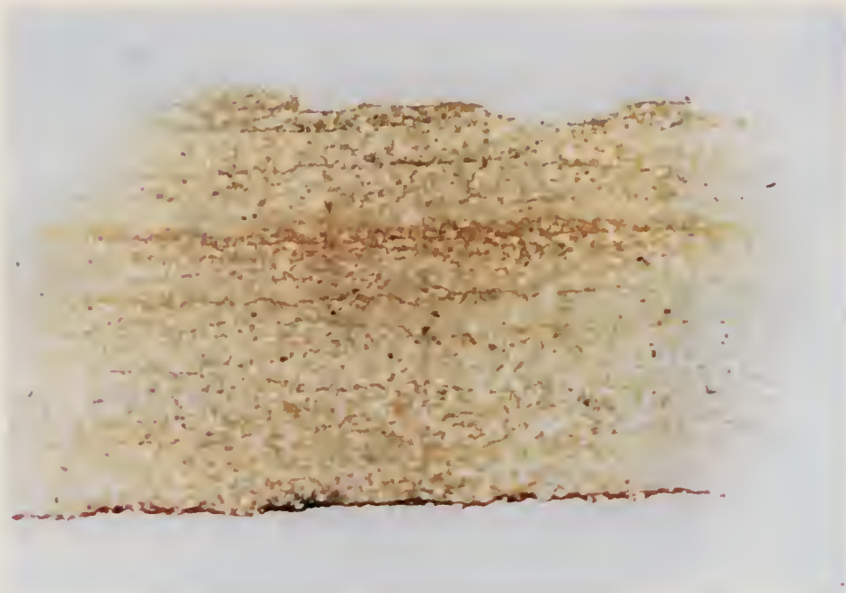
Fig. 28 Thin Section of Plaster from Kiva C from the Red Dado
