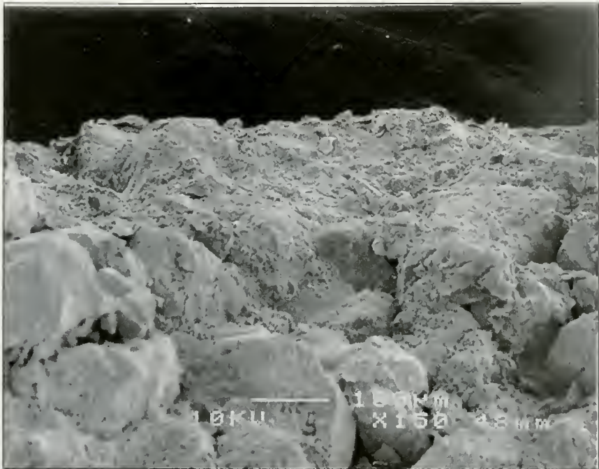
Fig. 43 - Honed surface (150X - JEOL SEM).
