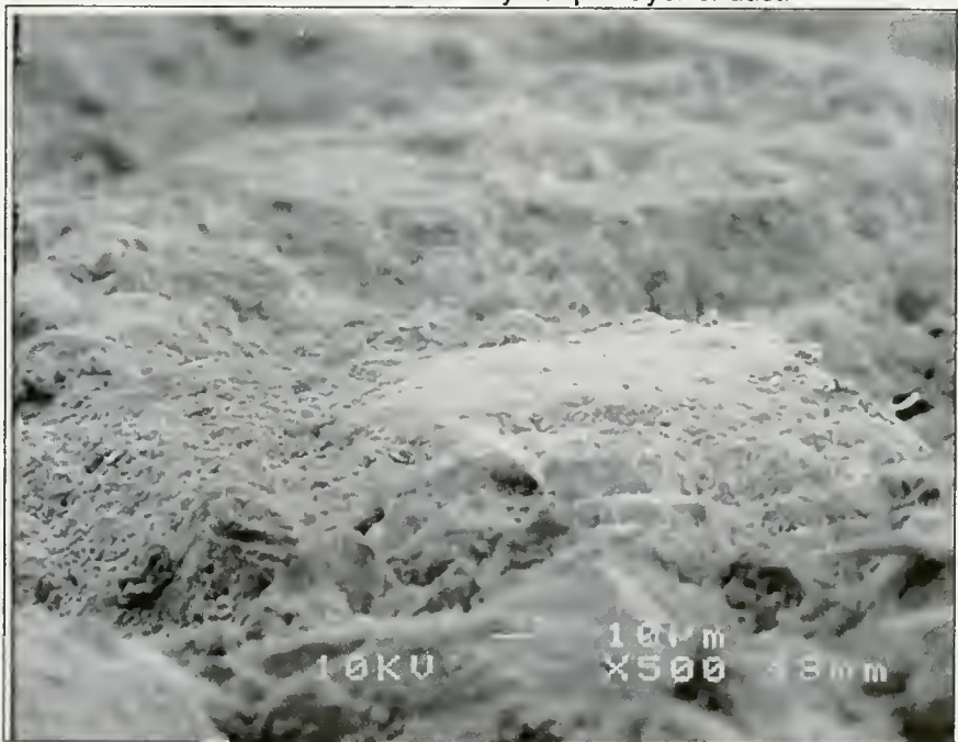
Fig. 59 - Honed Bethesda Terrace sandstone (500X – JEOL SEM). Dust layer completely covers sandstone grains.
