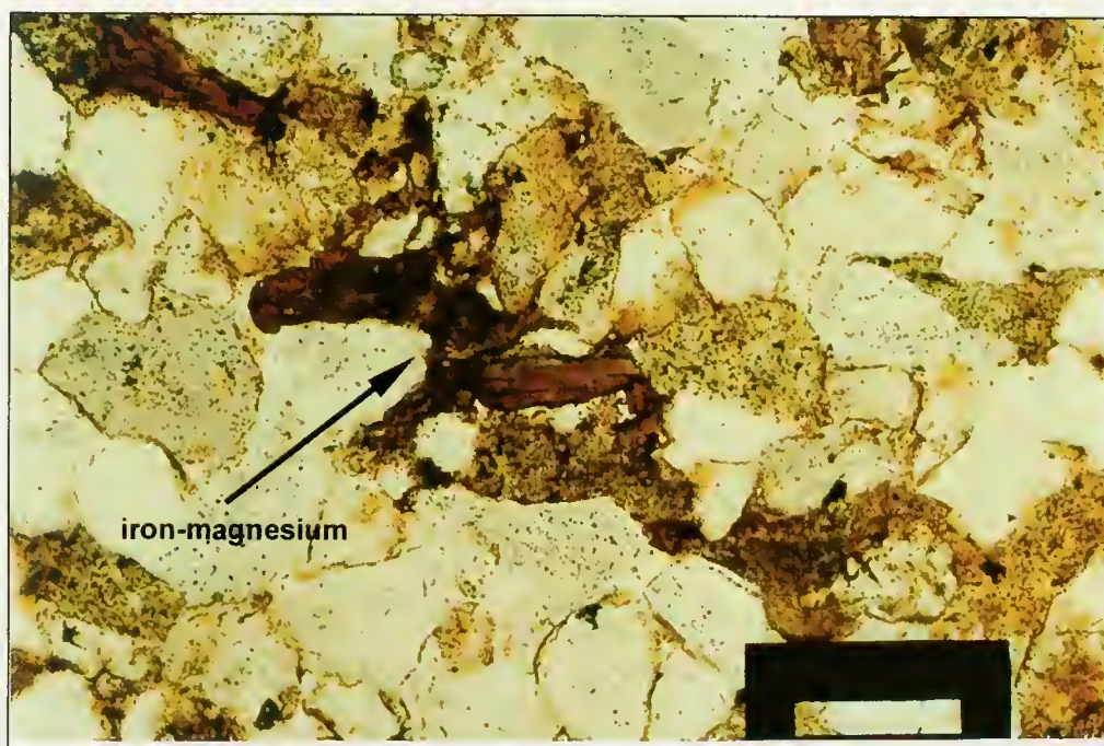
Fig. 33 - Bethesda Terrace sandstone (100X – plane-polarized light). Large inclusion of iron-magnesium in highly altered state.
