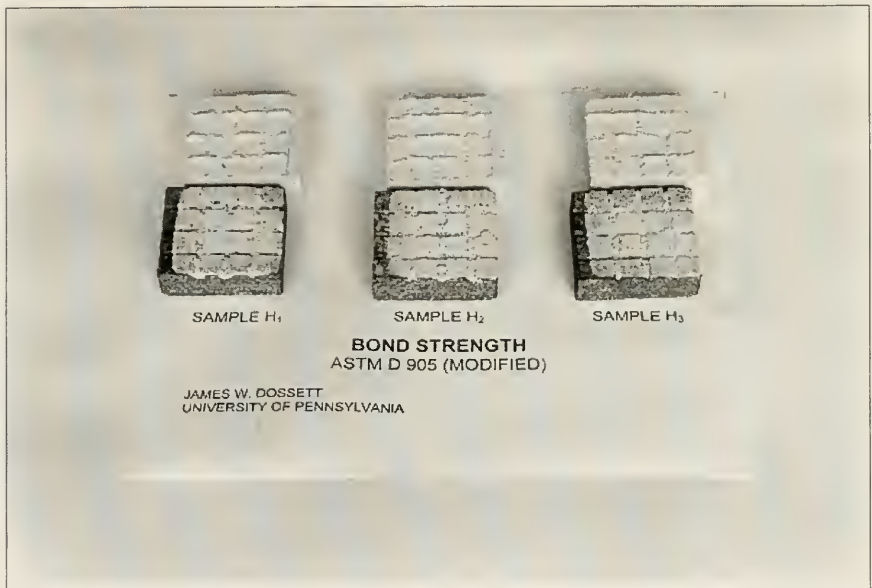
Figure 63 Bond Strength Test Sample H. There is a clean break at the bond line with no stone loss. About 45 % of the mortar originally in the grooves is retained on the mortar. Again note the direction of the retained grooved mortar - parallel to the direction of shear. There was good coverage.
