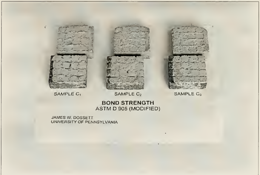
Figure 58 Bond Strength Test Sample C. There is a clean break at the bond line with no stone loss. About 10 % of the mortar originally in the grooves is retained on the mortar. There was good coverage during molding except for one small void ( 2 \text{ mm}^2 ) near the center of each replicate. This was probably caused by air pockets not removed by tamping.
