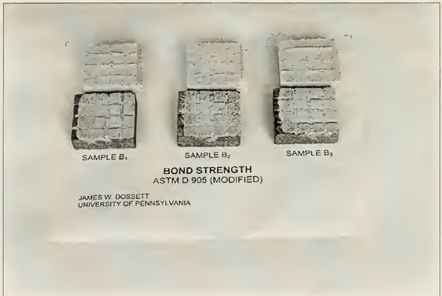
Figure 57 Bond Strength Test Sample B. There is a clean break at the bond line with no stone loss. About 25 % of the mortar originally in the grooves is retained on the mortar, indicating that the Acryl® 60 improved the cohesive strength of the mortar. There was good coverage during molding.
