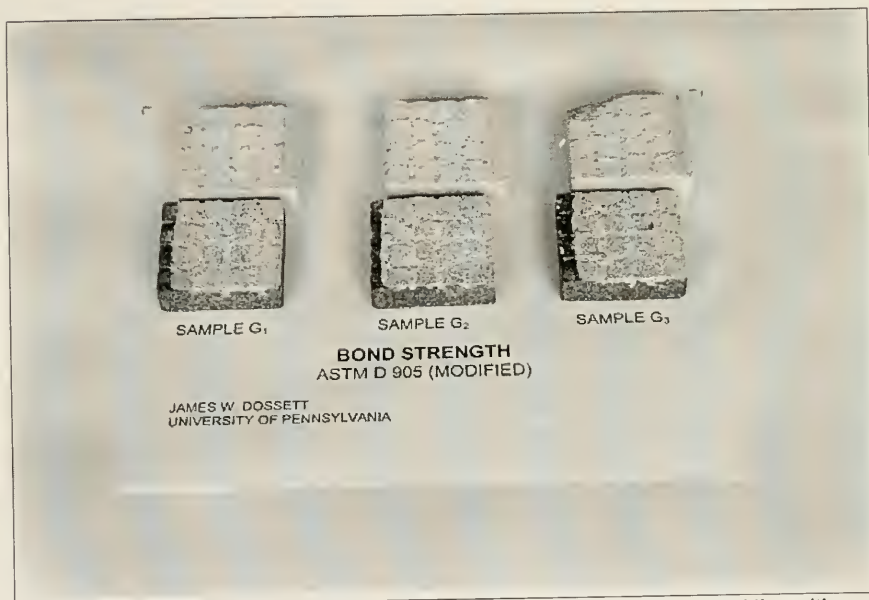
Figure 62 Bond Strength Test Sample G. There is a clean break at the bond line with no stone loss. About 10 % of the mortar originally in the grooves is retained on the mortar. The corner of the mortar in replicate 3 was dislodged during the test. There was good coverage.
