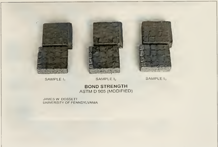
Figure 64 Bond Strength Test Sample I. This sample set has the most difference between replicates. Replicate 1 broke cleanly at the bond line with almost none of the mortar in the grooves retained on the mortar. Replicate 2 broke mostly at the bond line but left 25% of the stone surface still covered with mortar indicating that the bond strength was greater than the cohesive strength of the mortar. Replicate 3 left 10% of the stone still covered with mortar.
