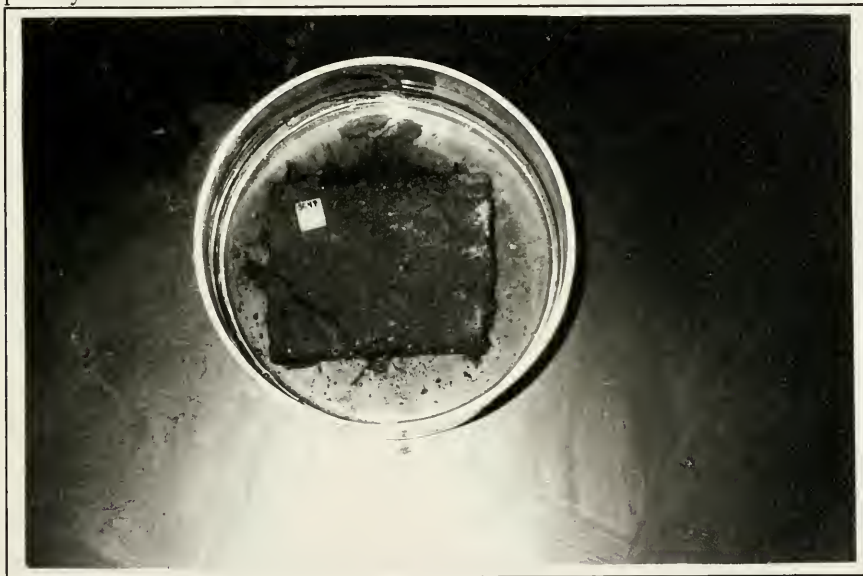
Figure 13. Salt Damaged Brick Sample Treated With B-67/Silane Consolidant After Two Hour Soak. This degree of damage was typical of Type 1 salt damaged samples treated with both the acrylic and epoxy resin consolidants.
