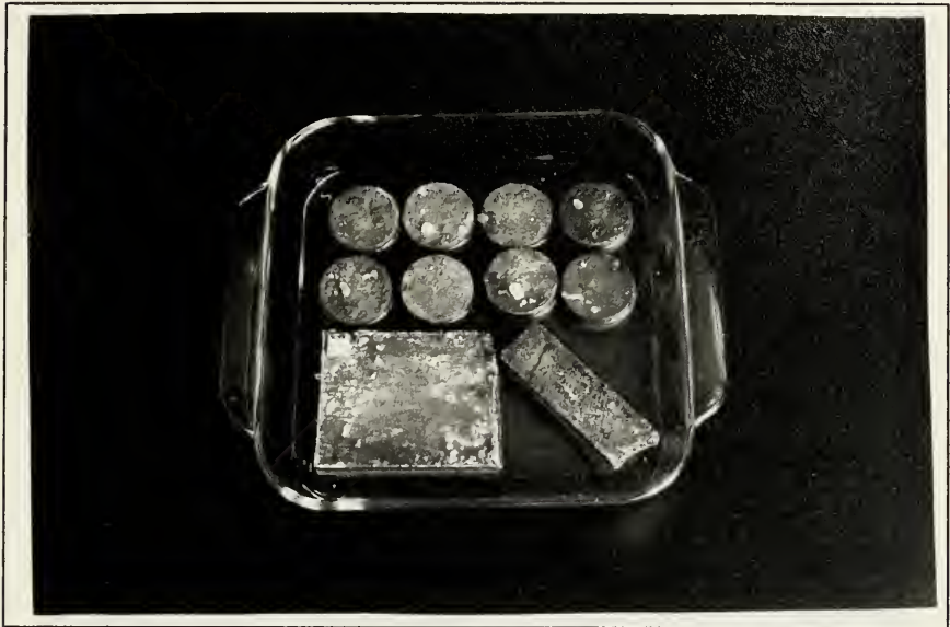
Figure 14. Samples Disks soaking in Epoxy Resin/Silane Consolidant in Preparation for Water Vapour Transmission Test.
