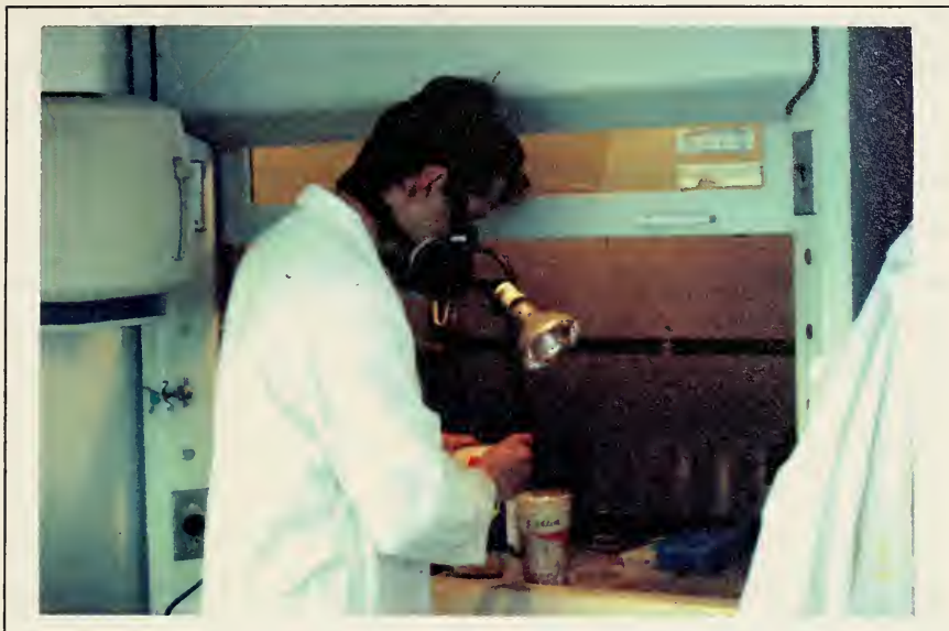
Figure 12. Mixing the Epoxy Resin /Silane Consolidant under a Fume Hood while wearing a respirator.
