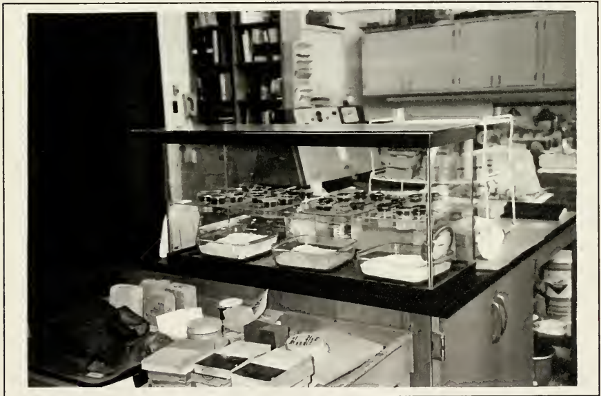
Figure 15. Water Vapour Transmission Tank During Testing of Brick Disks.
