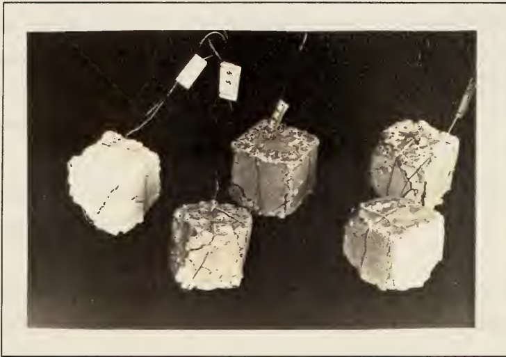
Photo 7 - Samples after 10 cycles of 14% solution sodium sulphate crystallization test, note the cracking of the cubes and salts on the surface of the cubes.
