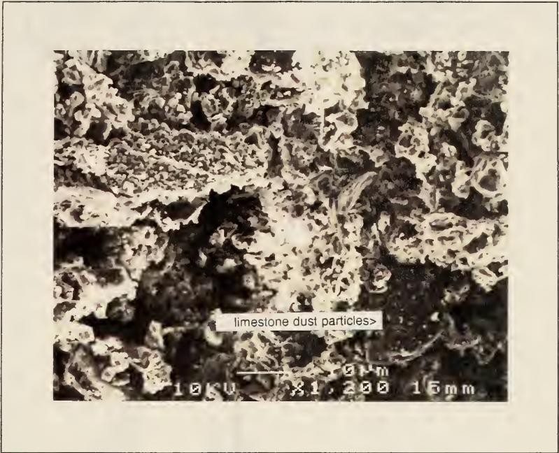
Photo 17 - SEM microphotograph, Mag x1200, Mix 4 (1 part lime, 2.5 parts sand and 1 part limestone dust)
