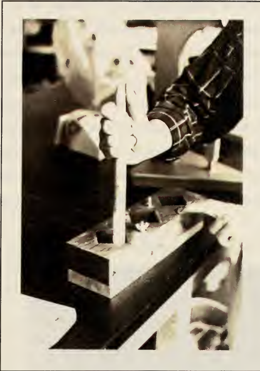
Photo 1 - Tamping with a non-absorptive, non-brittle tamper into the 50mm or 2 in Wooden Cube mold.
