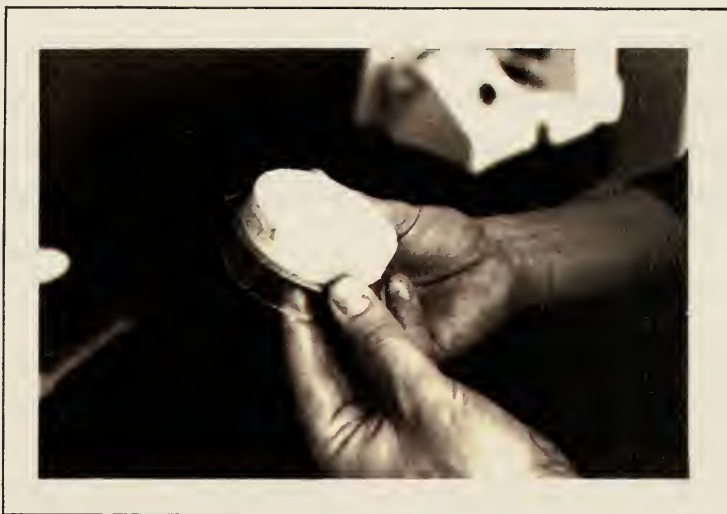
Photo 3 - Sample being demolded from PVC ring mold.
