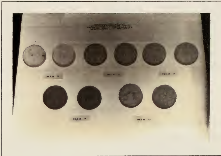
Photo 6 - Samples after 12 cycles of 10% solution sodium sulphate crystallization test
