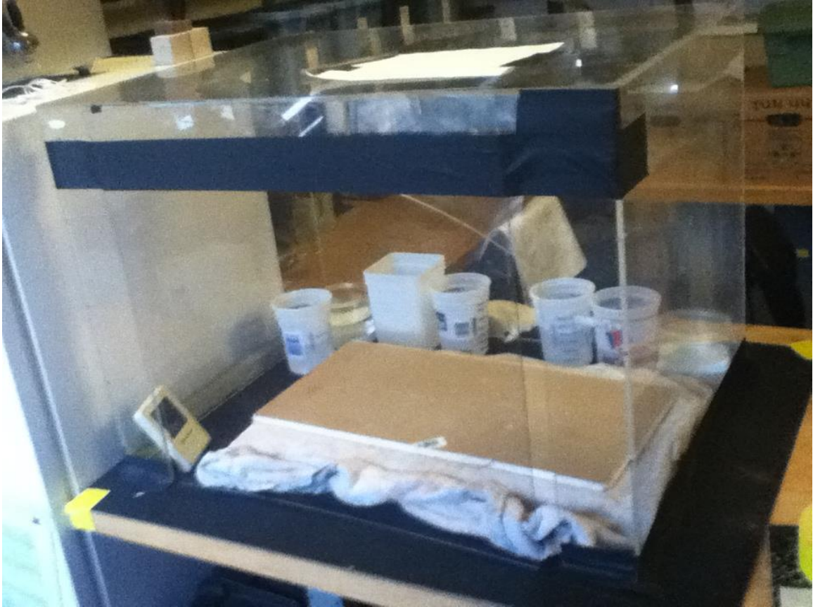
Figure 5.1 Humidity chamber. Photo taken by author, 2013.
