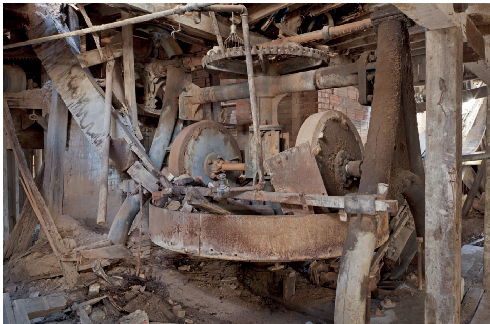
Figure 3.10: Western Clay dry pan. Joe E. B. Elliott, photographer, July 2011. Courtesy of the University of Pennsylvania Architecture Conservation Laboratory.
