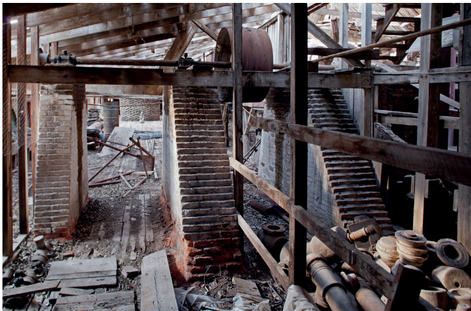
Figure 3.8: Western Clay's line shaft and belts in relation to the tile shop drying room (in background). Joe E. B. Elliott, photographer, July 2011. Courtesy of the University of Pennsylvania Architecture Conservation Laboratory.
