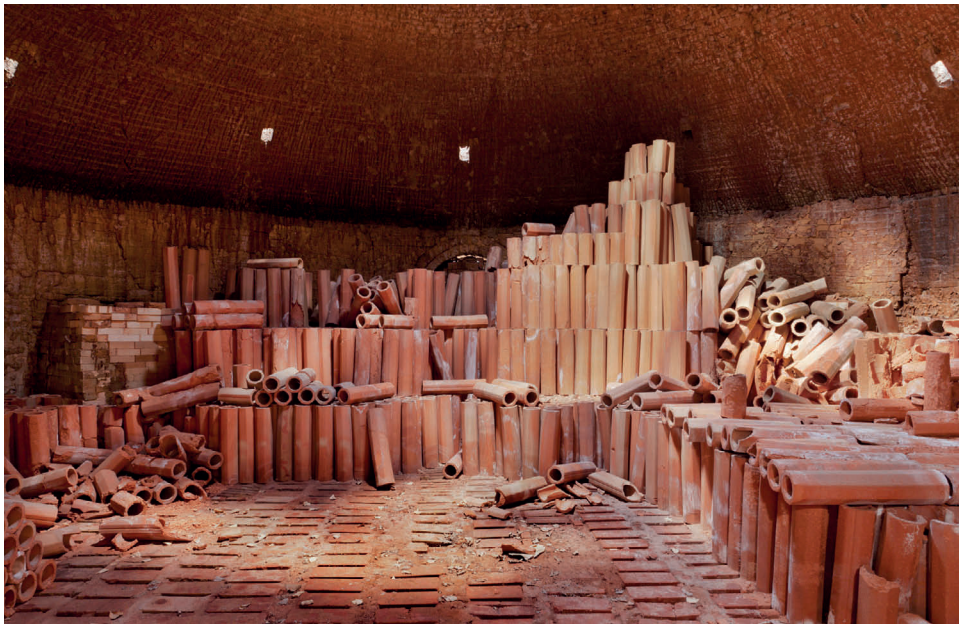
Figure 3.16: Western Clay kiln "Number 8," stacked with drain pipe. Joe E. B. Elliott, photographer, July 2011. Courtesy of the University of Pennsylvania Architecture Conservation Laboratory.
