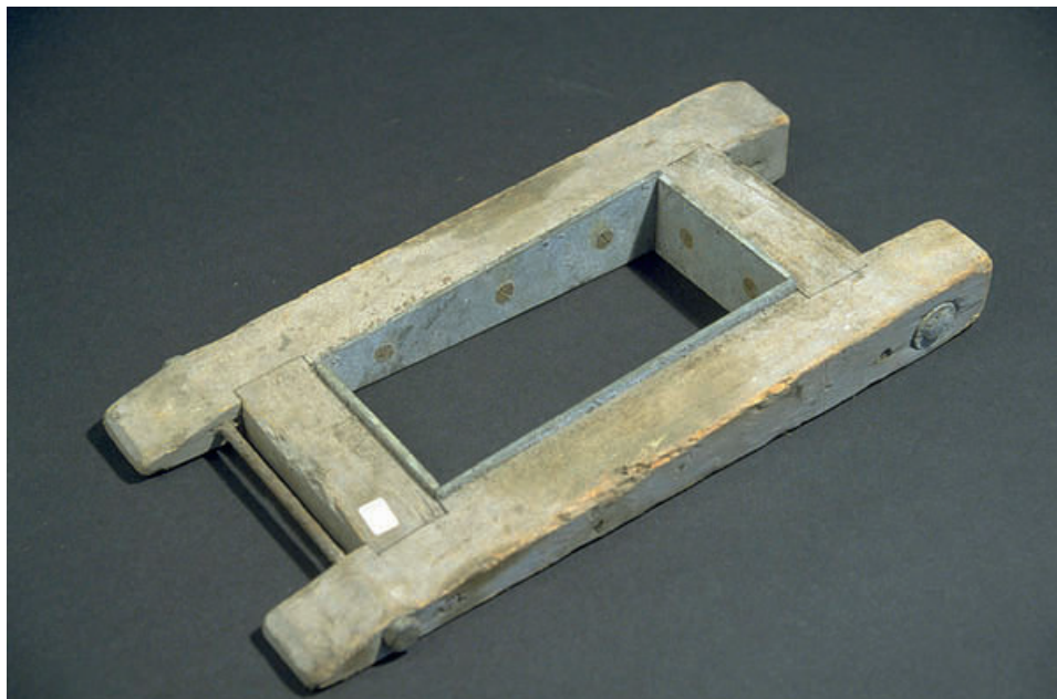
Figure 2.11: "Wood and Steel Brick Mould." Photographer unknown, 2007. Courtesy of the East Lothian Museum, East Lothian, United Kingdom. Image from http://www.flickr.com/photos/eastlothian/540650616/in/photostream/lightbox/ .
