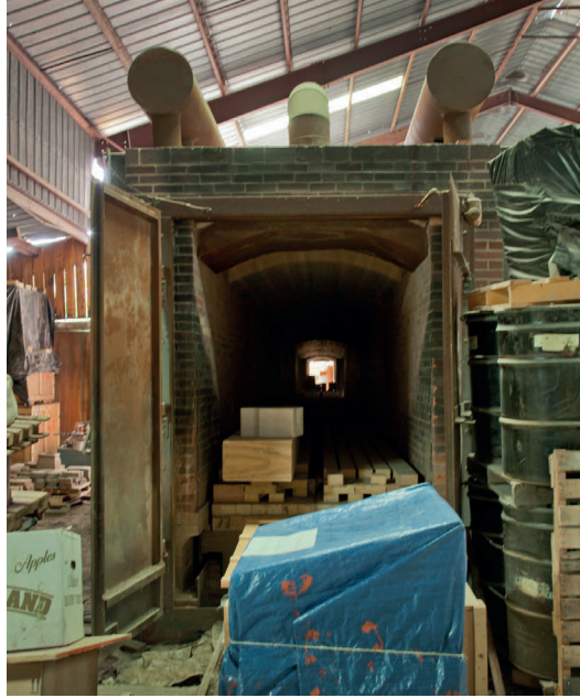
Figure 2.22: Remains of the late 1950's Tunnel Kiln at Western Clay. Joe, E. B. Elliott, photographer, July 2011.
