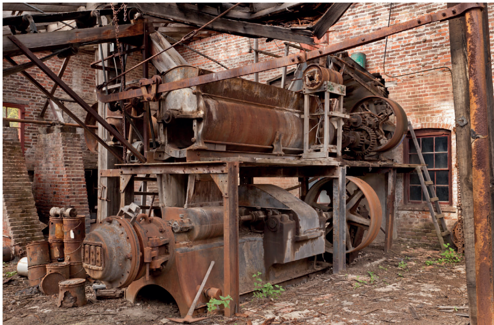
Figure 2.35: Western Clay tile shop pug mill. Joe E. B. Elliott, photographer, July 2011. Courtesy of the University of Pennsylvania Architecture Conservation Laboratory.
