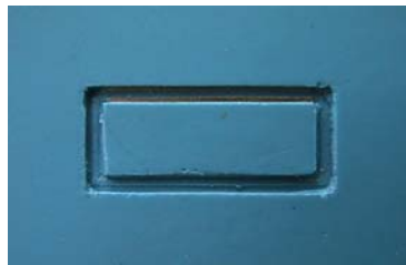
Fig. 5: A rectangular loop fabricated in LTCCs. Electrodes were printed only along the upper conduit.
