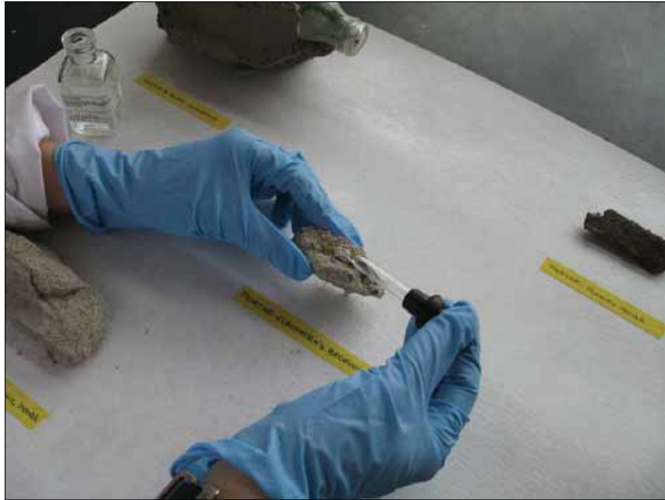
Figure 7.11: Phenolphthalein test for carbonation of mortar. (L. Hall 2007)
