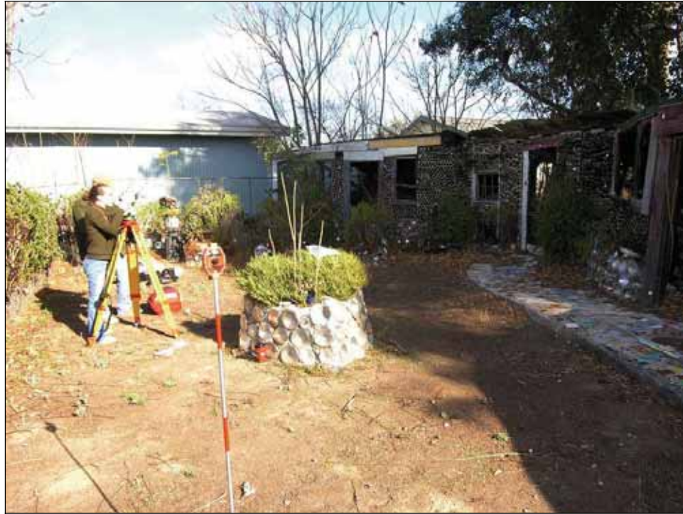
Figure 6.1: Data collection with a REDM Leica TCR 307. (GCI 2007)
