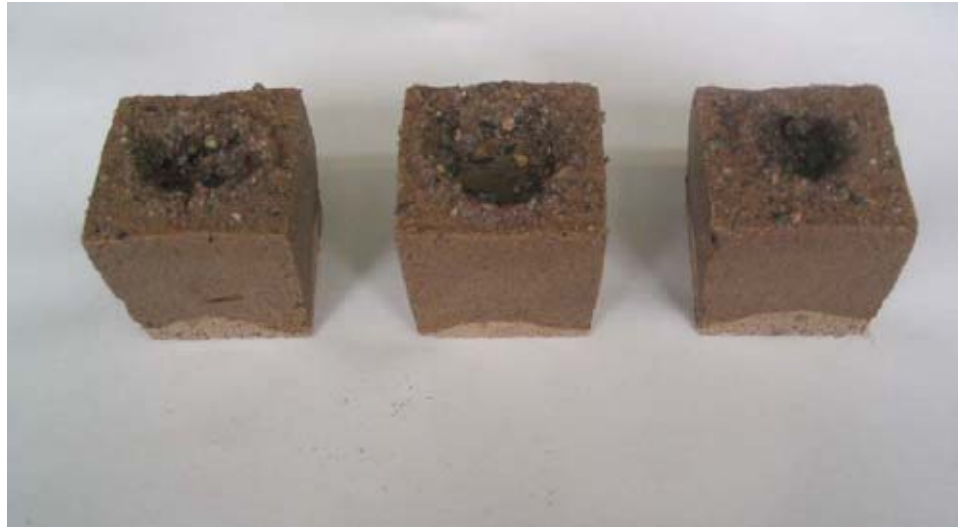
Figure I3. Unamended samples of Bandelier soil (Garcia Landscape Materials blend) displayed an average penetration depth of 20.61 mm following 1 hour of exposure to falling water droplets.
