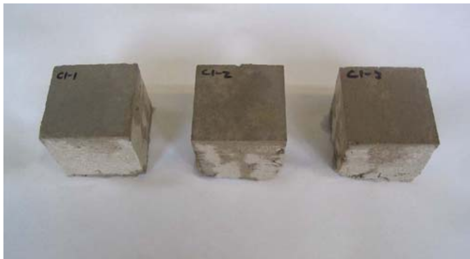
Figure I4. Formulation C1 samples following 1 hour of exposure to falling water droplets displayed no evidence of penetration on exposed surfaces.
