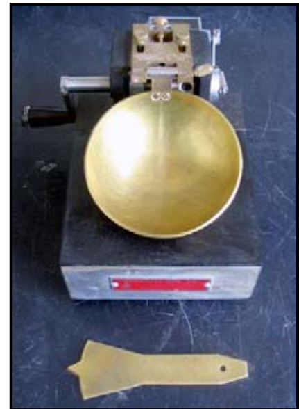
Figure 3.3. Casagrande device with grooving tool.
