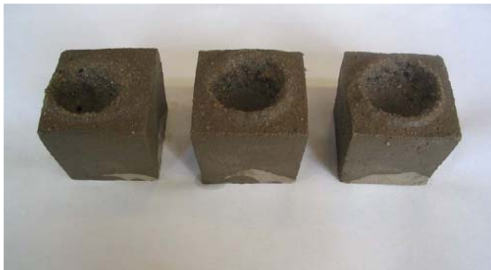
Figure 16. Unamended samples of Chaco soil (BLM quarry) displayed an average penetration depth of 15.04 mm following 1 hour of exposure to falling water droplets.
