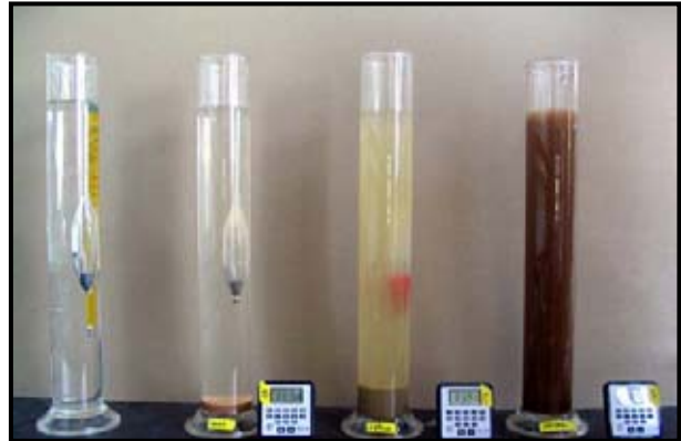
Figure 3.2. Soil sedimentation cylinders with control cylinder on left.
