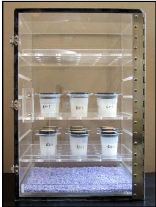
Figure 3.10. Climate-controlled chamber with vapor transmission assemblies.
