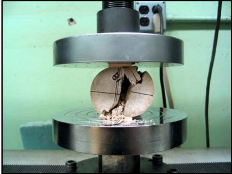
Figure 3.13. Sample failing under compression.
