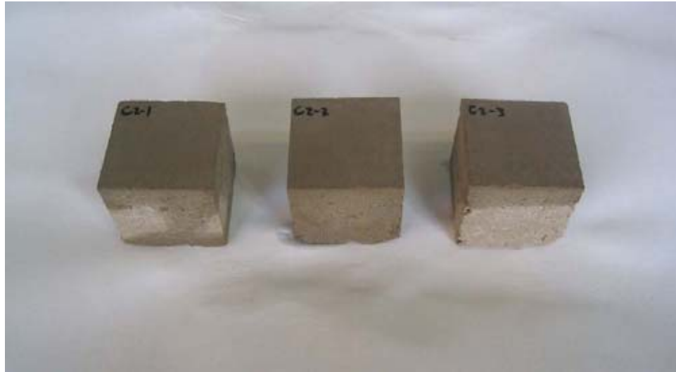
Figure 15. Formulation C2 samples following 1 hour of exposure to falling water droplets displayed no evidence of penetration on exposed surfaces.
