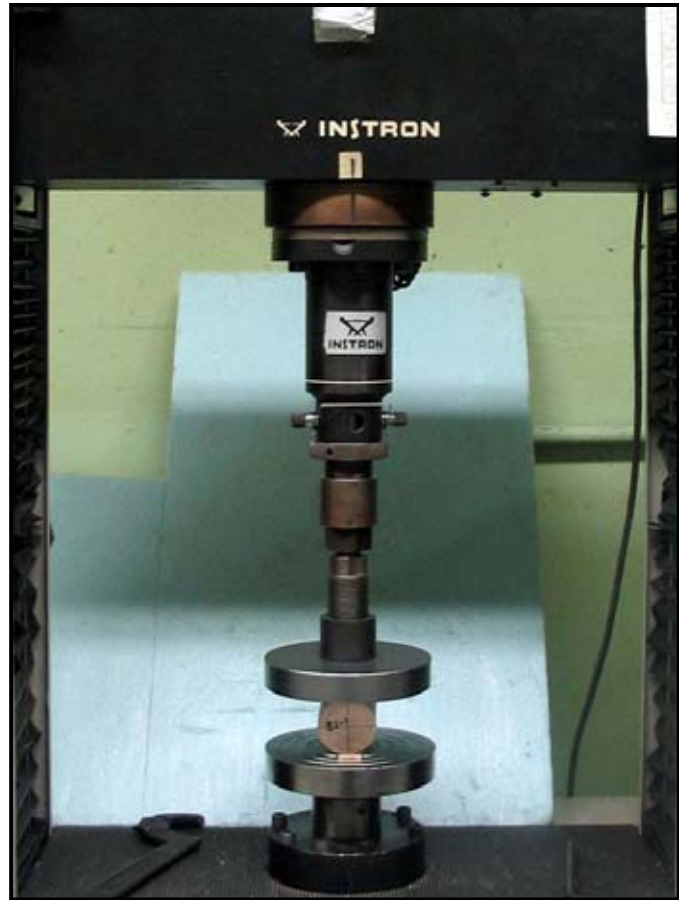
Figure 3.12. Instron Model 4206 set for compression.
