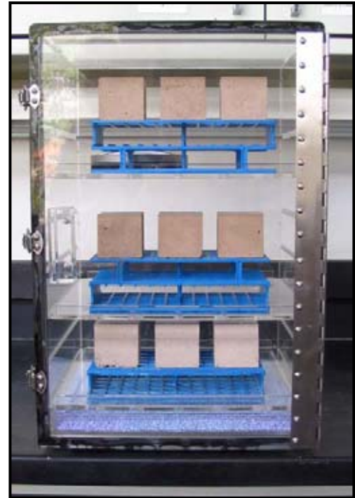
Figure 3.8. Climate-controlled chamber containing drying index samples.
