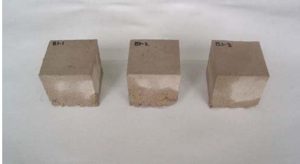
Figure I1. Formulation B1 samples following 1 hour of exposure to falling water droplets displayed no evidence of penetration on exposed surfaces.
