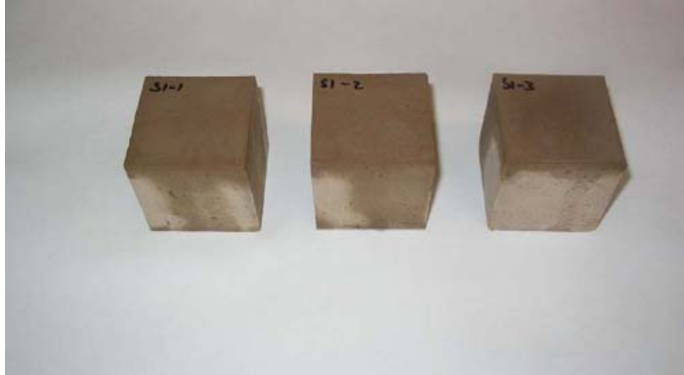
Figure I7. Formulation S1 samples following 1 hour of exposure to falling water droplets displayed no evidence of penetration on exposed surfaces.
