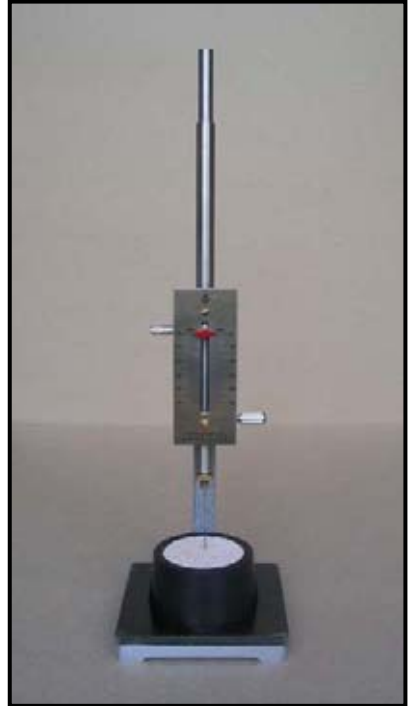
Figure 3.6. Vicat Apparatus with ring mold and sample.
