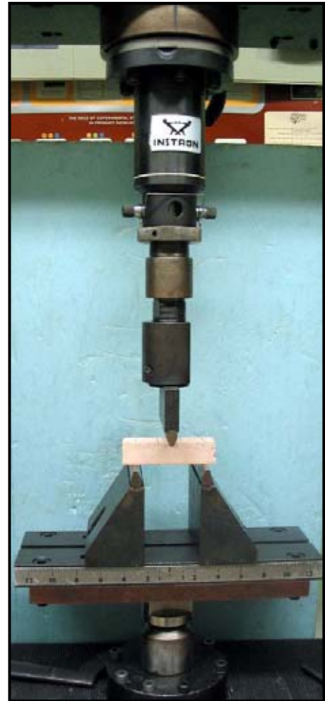
Figure 3.13. Instron Model 4206 set for three-point bending.
