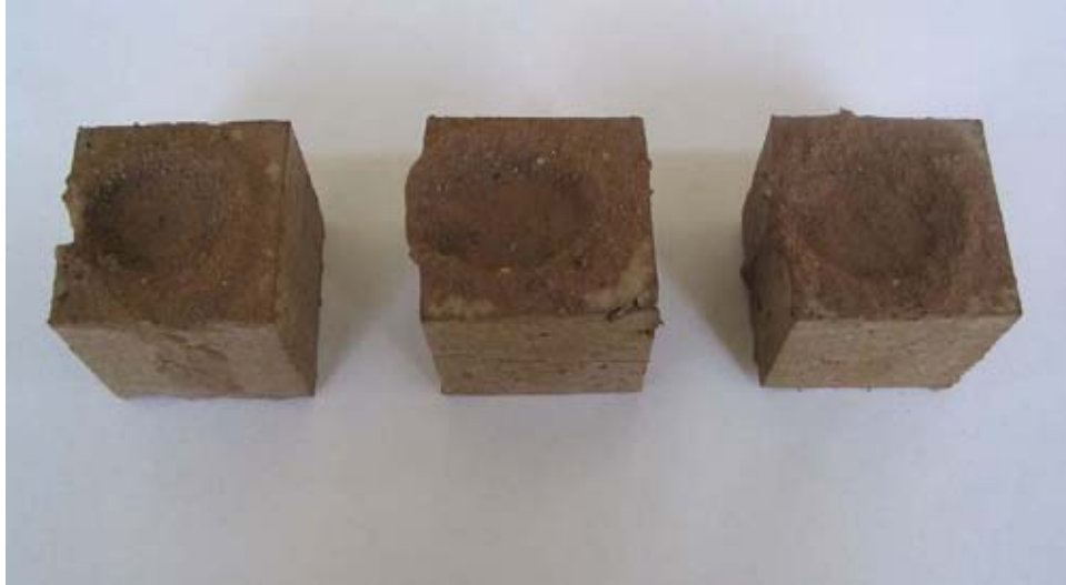
Figure 19. Unamended samples of Salinas soil (local quarry) displayed an average penetration depth of 8.75 mm following 1 hour of exposure to falling water droplets.
