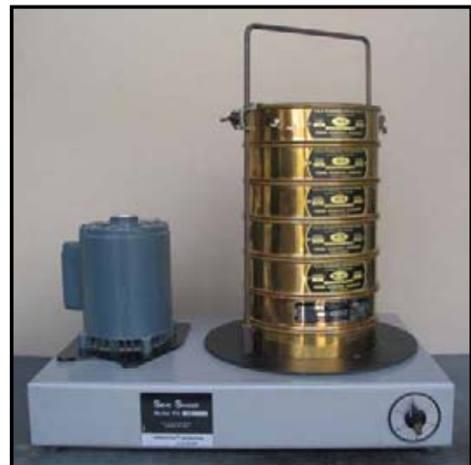
Figure 3.1. ASTM sieve stack and mechanical sieve shaker.
