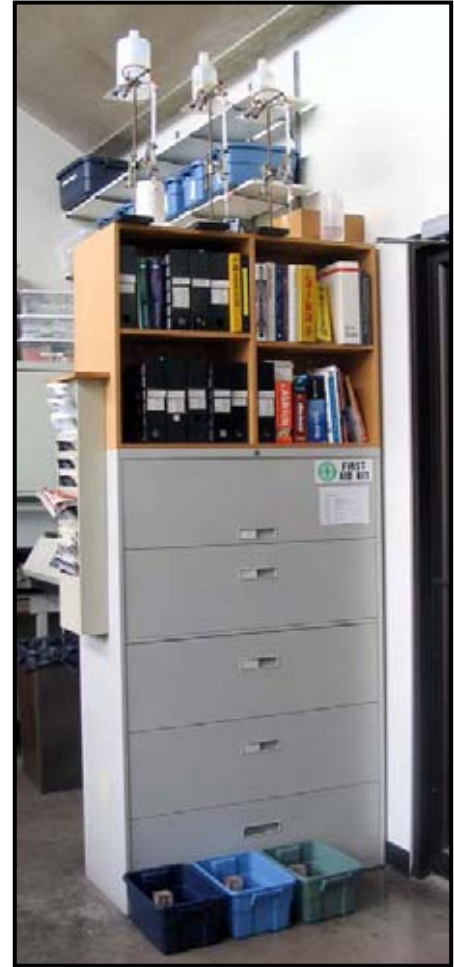
Figure 3.12. CRATerre Water Drop Erosion test array in operation in the Architectural Conservation Laboratory
