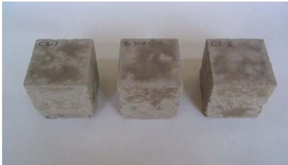
Figure I8. Formulation C2 samples photographed after fifteenth freeze/thaw cycle showing no visible deterioration.
