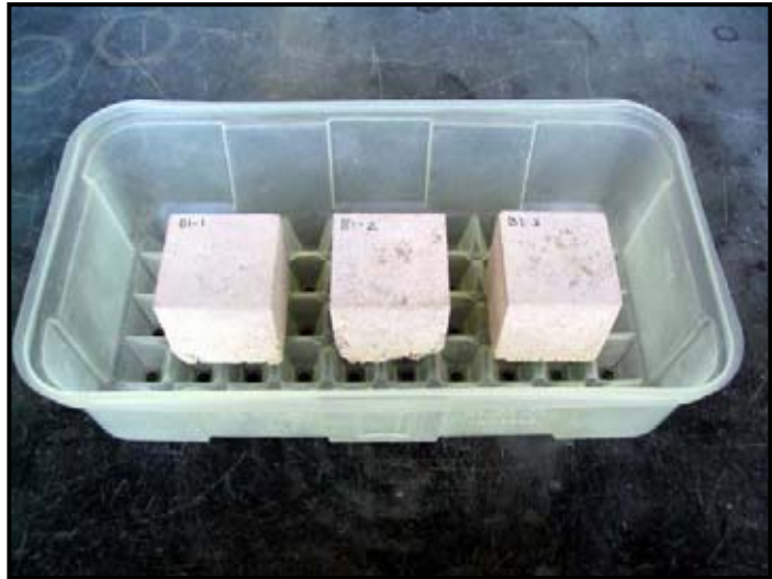
Figure 3.9. Frost resistance specimens in raised-bottom tray.
