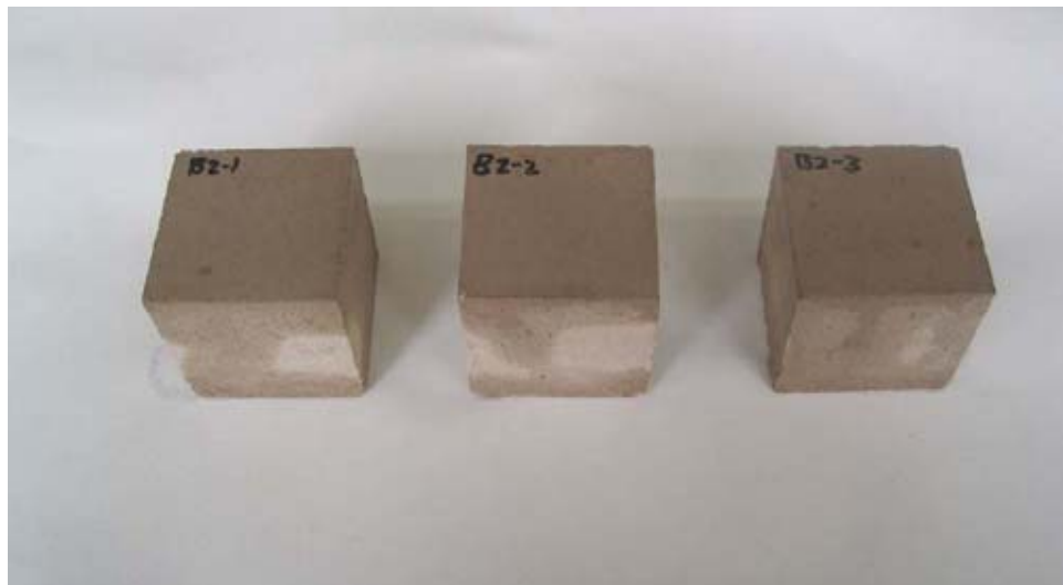
Figure I2. Formulation B2 samples following 1 hour of exposure to falling water droplets displayed no evidence of penetration on exposed surfaces.
