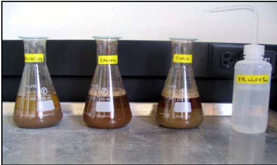
Figure 4.1 Soil samples submerged in 3% sodium hydroxide solution.
