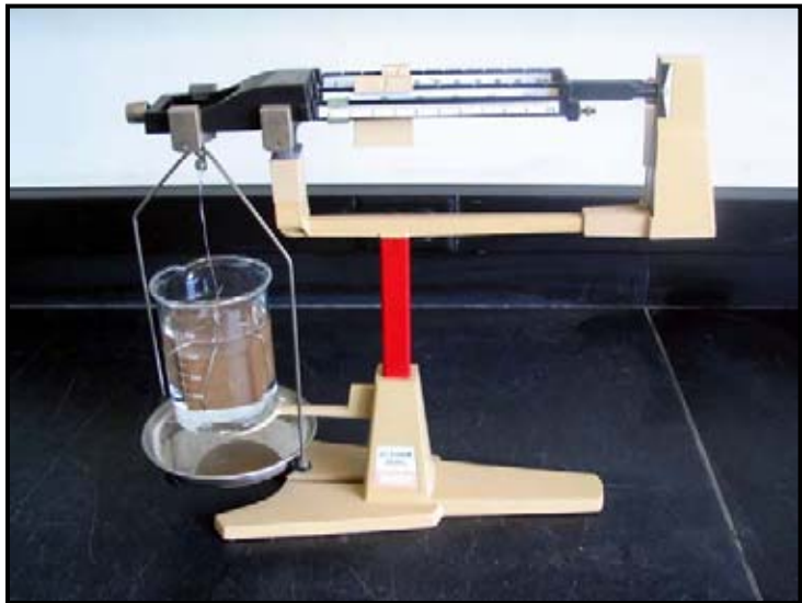
Figure 3.7. Triple-beam balance for hydrostatic weighing of samples.
