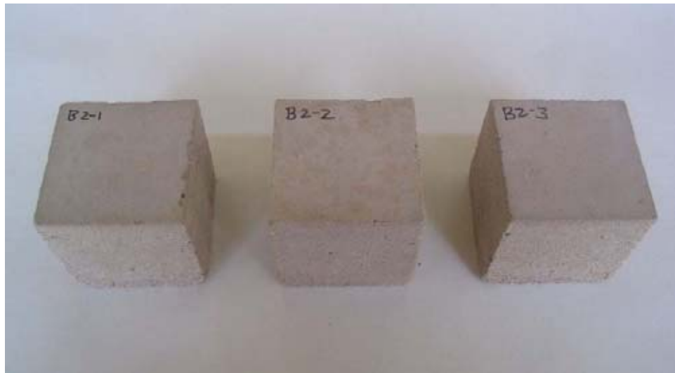
Figure I4. Formulation B2 samples photographed after fifteenth freeze/thaw cycle showing no visible deterioration.
