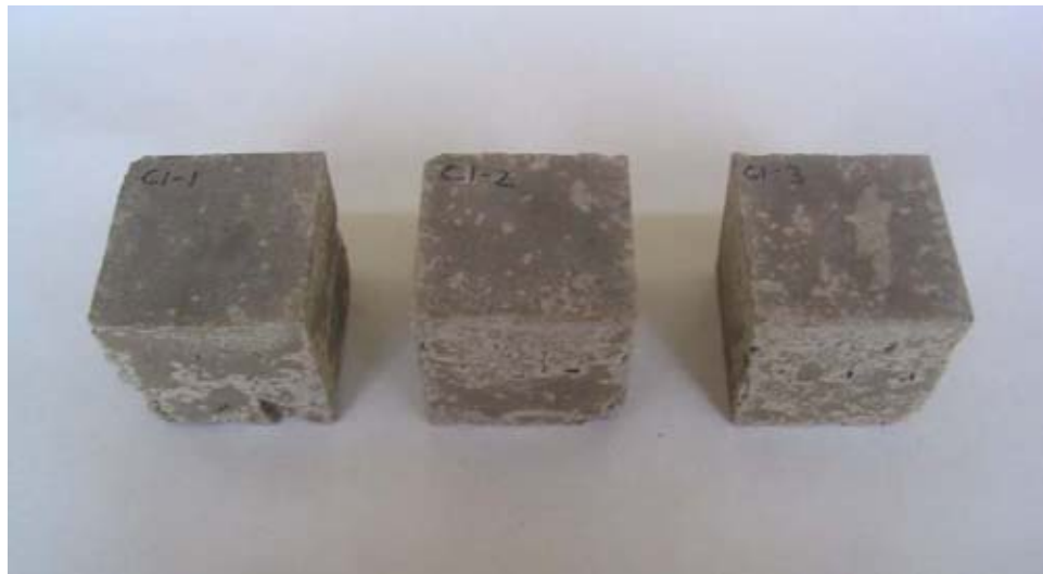
Figure I6. Formulation C1 samples photographed after fifteenth freeze/thaw cycle showing no visible deterioration.
