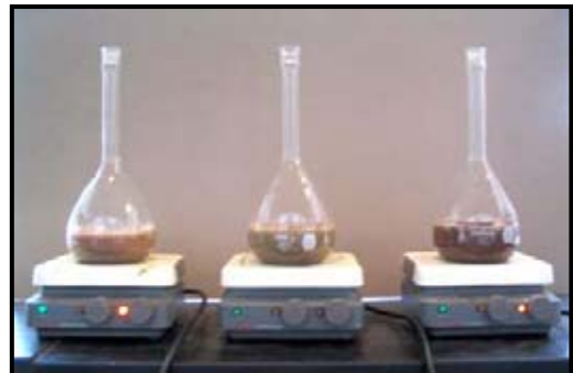
Figure 3.4. Soil slurries during deairation.
