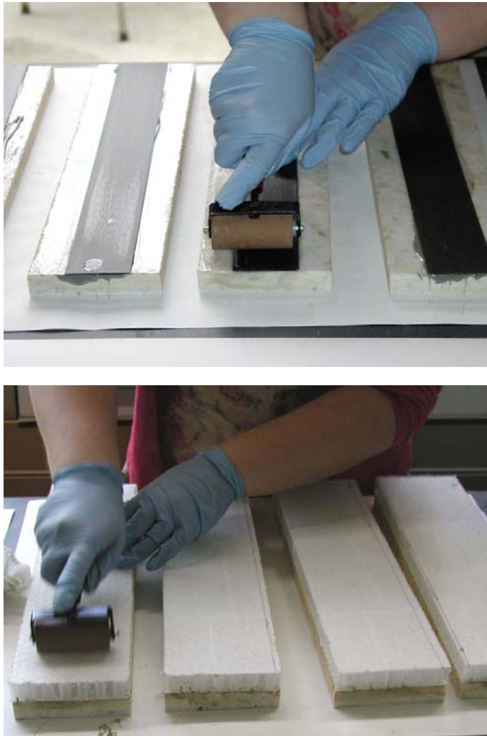
Figure 3.7 Step four: Roll the carbon fiber strap or the polypropylene honeycomb over the epoxy to ensure even contact.
