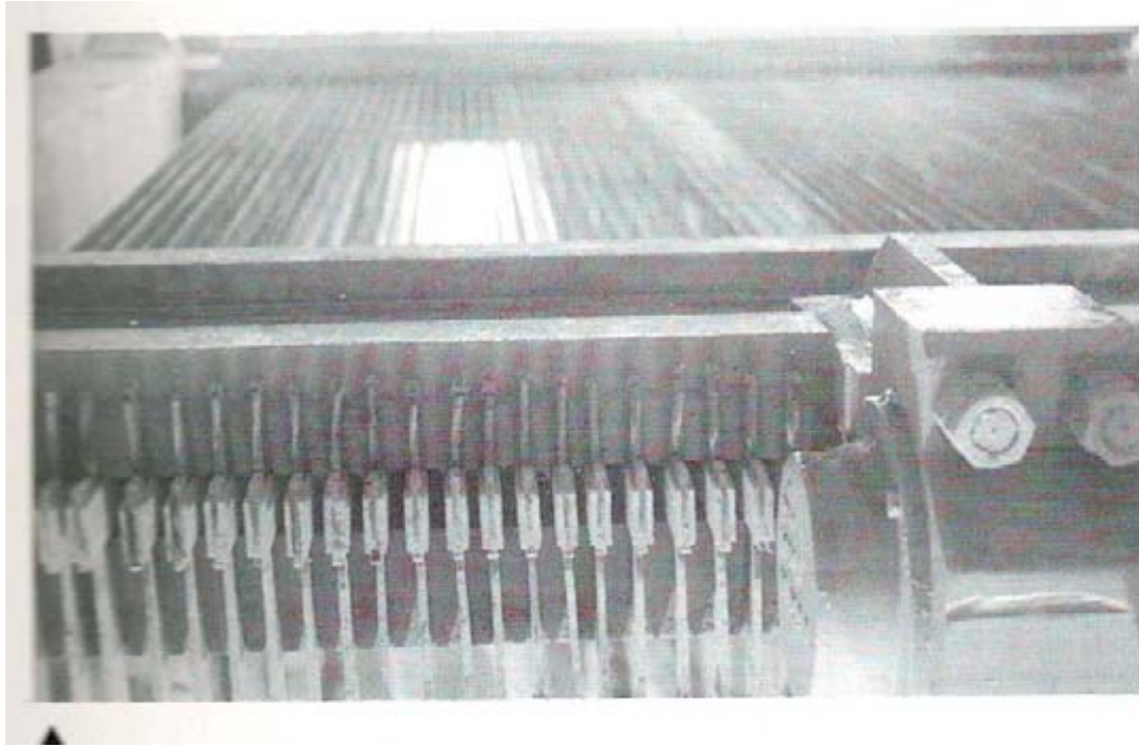
Figure 1.1 Multi-bladed gang saw. (Photo from Lewis, 19.)
