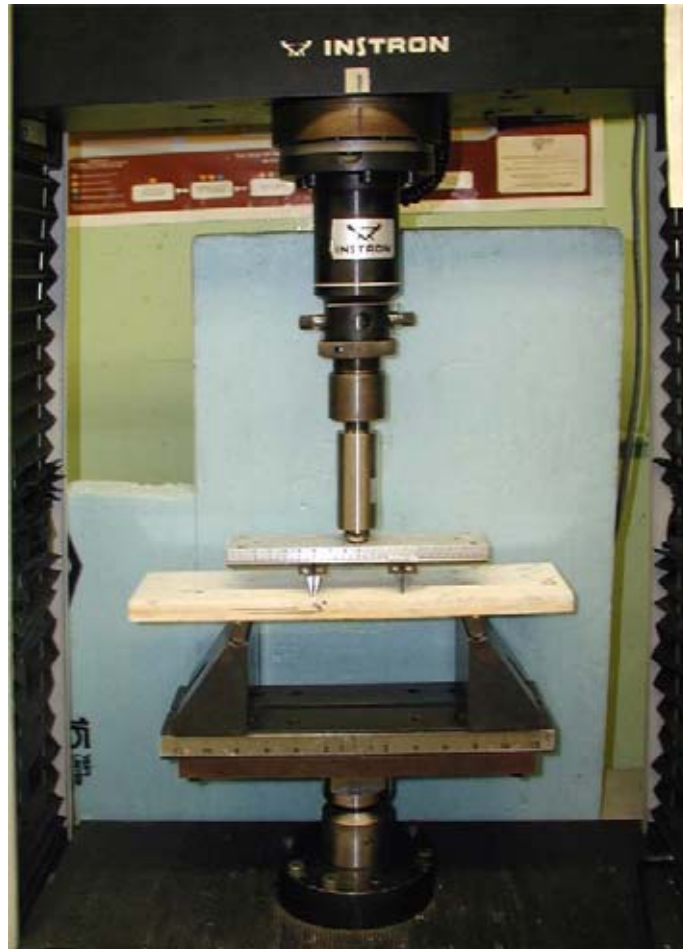
Figure 3.12 Flexural strength, quarter-point loading Instron test assembly.
