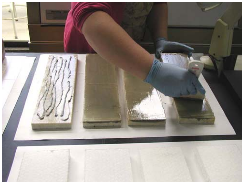
Figure 3.5 Step two: Spread the epoxy over the marble panel.
