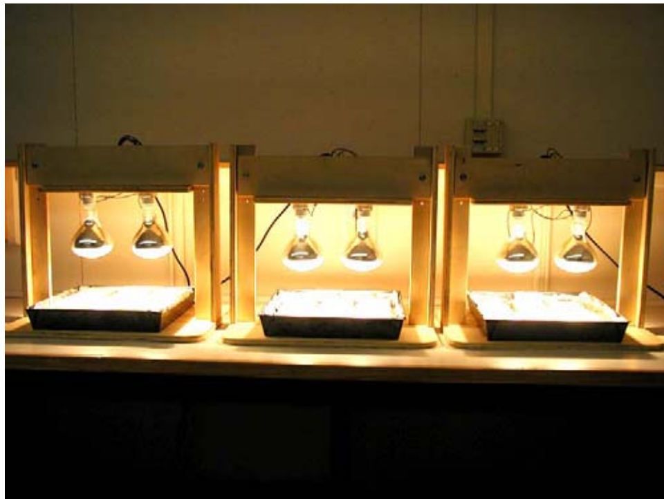
Figure 3.8 Constructed bowing potential assemblies.
