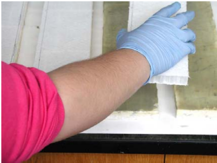
Figure 3.6 Step three: Apply treatments to the marble on top of the epoxy.
