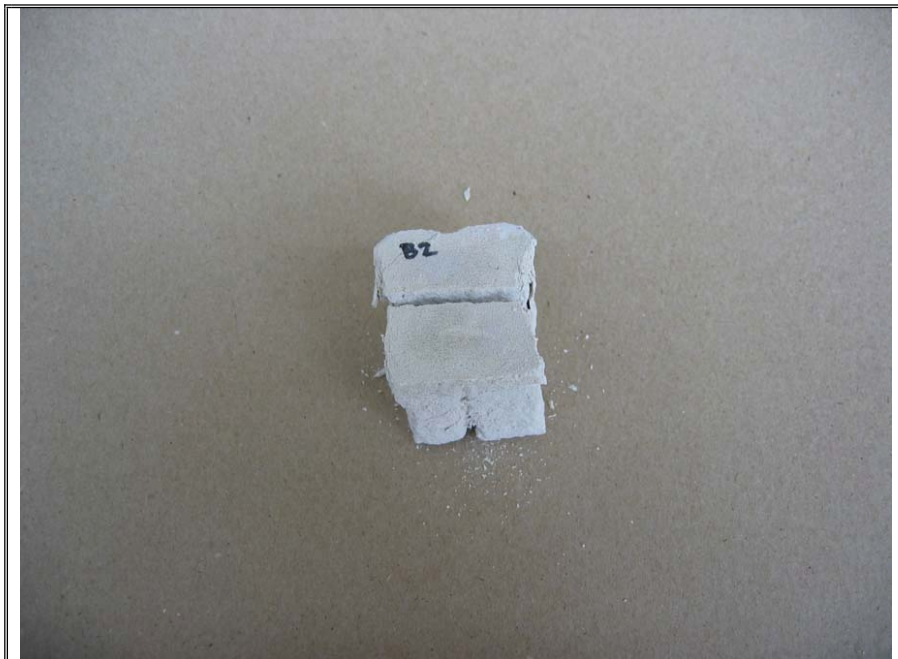
Sample B2 after 12 immersion cycles in 10% sodium sulfate solution, 7-day immersion in tap water, and drying in oven. B1 and B3 failed after the 10 th cycle after cracking in half. B1 exhibited significant disaggregation around its center.
