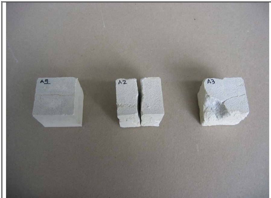
Sample Group A after 14 immersion cycles in 10% sodium sulfate solution, 7-day immersion in tap water, and drying in oven. A1 has visible cracks, A2 is split vertically, and A3 exhibits notable erosion and cracking.
