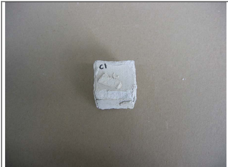
Sample C1 after 14 immersion cycles in 10% sodium sulfate solution, 7-day immersion in tap water, and drying in oven. C3 disintegrated after the 10 th cycle. C2 failed after the 12 th cycle.
