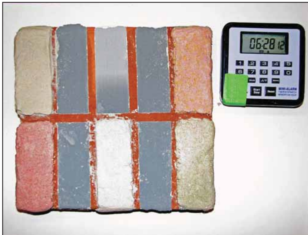
Figure 5.8: Used resins exposed after one hour (Source: C. Smith, 2009).
