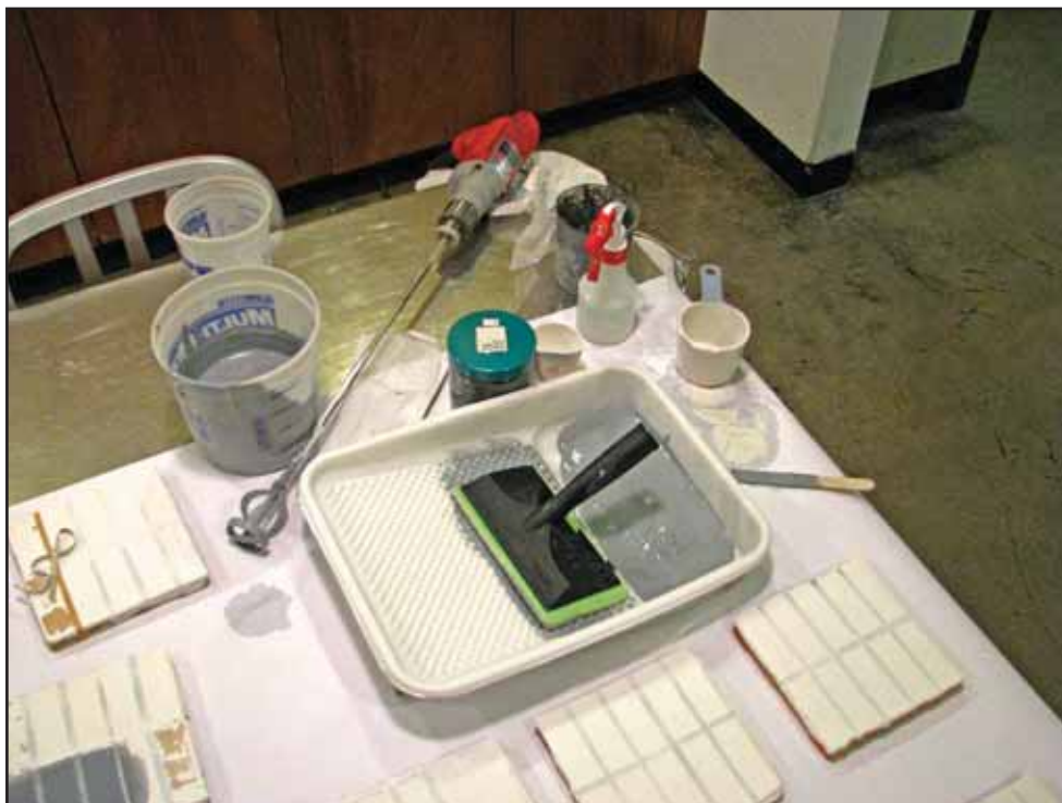
Figure 5.5: Materials used in sample preparation, including Polyken tape, terracotta tiles, limewash, drill, lamp black, and pad painter (Source: C. Smith, 2009).
