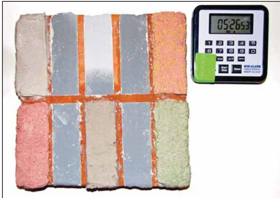
Figure 5.7: Tile covered with fresh resin formulations. Counterclockwise from bottom: C-211 H, control, C-211 Na, CNP 80, TP 207 (Source: C. Smith, 2009).
