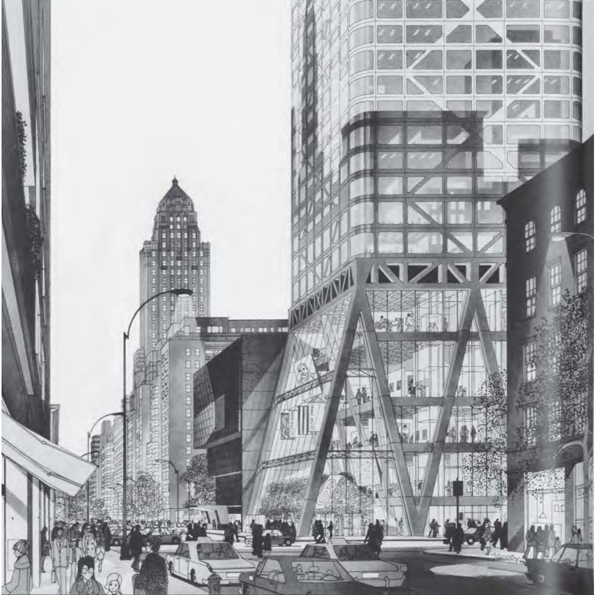
Fig. 75. Rendering - Whitney Museum Addition, Foster, 1978. The additional gallery floors accommodated by Foster's tower are visible in the middle-right, suspended within the triangulated atrium space. There are some nods to Breuer with the progressive cantilevering of the new gallery floors, and the gridded ceilings.
