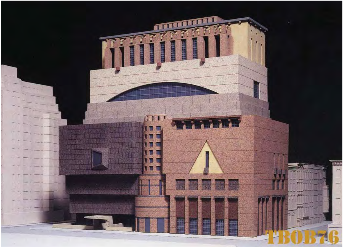
Fig. 76. Model - Whitney Museum Addition, Graves, 1985. This was Graves' first proposal, consisting of four parts: a stepped hinge, a new mass south of the Breuer building, and then a podium and temple-like structure immediately above.
