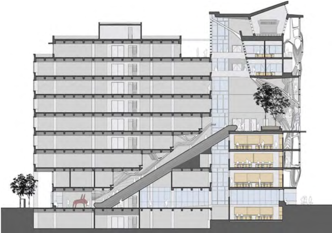
Fig. 54. Section - Building C and addition (designed 2005). Original building to left, with 28th Street to the right. A new escalator will maintain the existing building's entrance, and directly connect with a new multi-story student lounge. The fresnel system is located on the addition's south-facing elevation at top.
