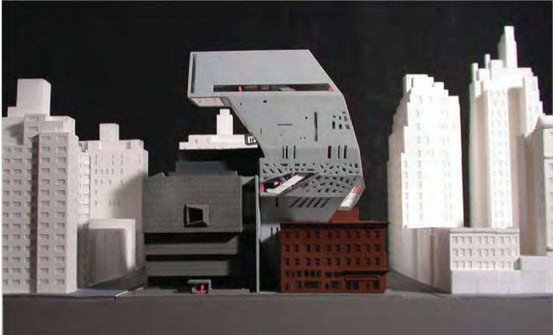
Fig. 84. Model - Whitney Museum Addition, Koolhaas, 2003. Koolhaas's scheme involved demolishing the northernmost Madison brownstone, then launching his addition out of the block's interior. The four remaining brownstones would become gallery space for prewar art.
