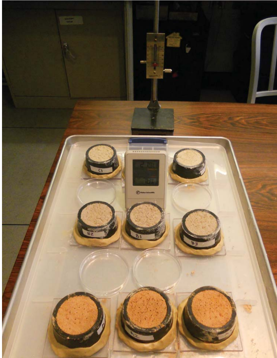
Figure 6.1: Setting time test samples in (uncovered) humidity chamber (Rogers)
