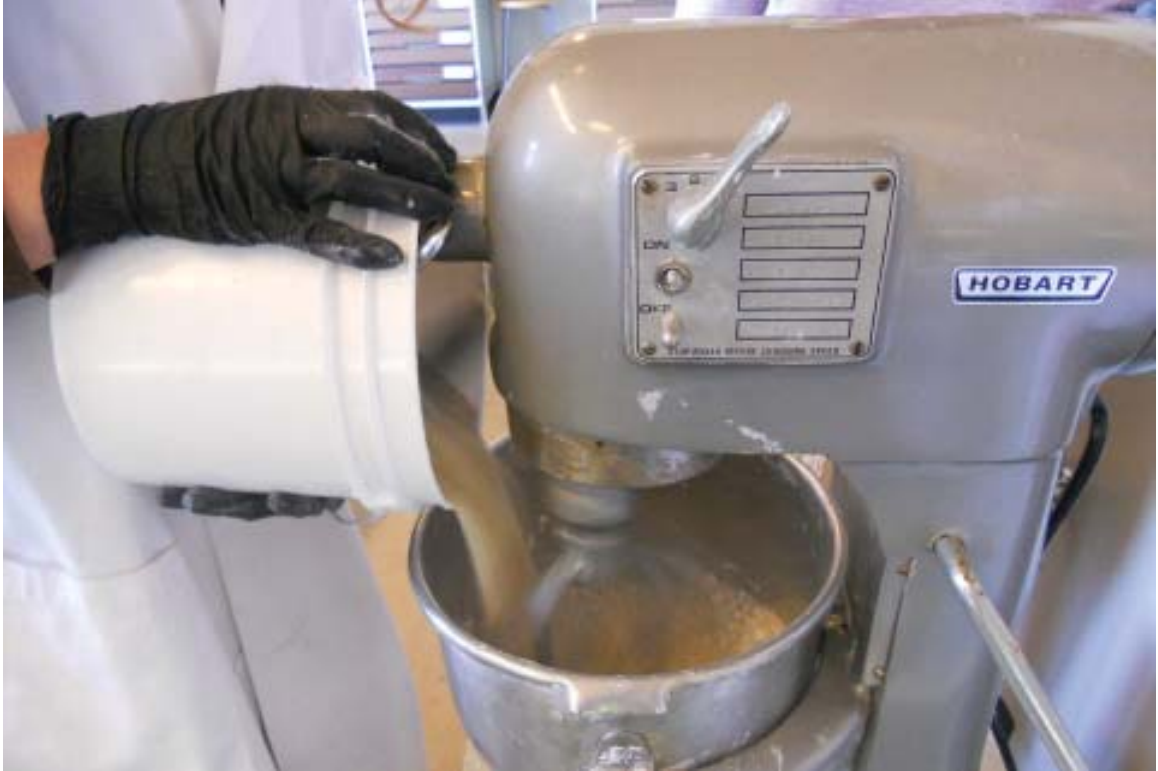
Figure 5.6: Mixing Formulation B using Hobart C-100 mixer (Rogers)
