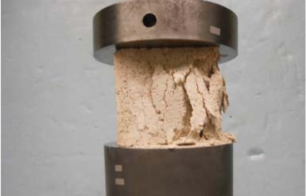
Figure 7.17: Compressive Strength Test, Formulation B mortar cube after crushing (Rogers)
