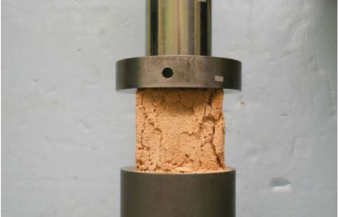
Figure 7.15: Compressive Strength Test, Formulation A mortar cube after crushing (Rogers)
