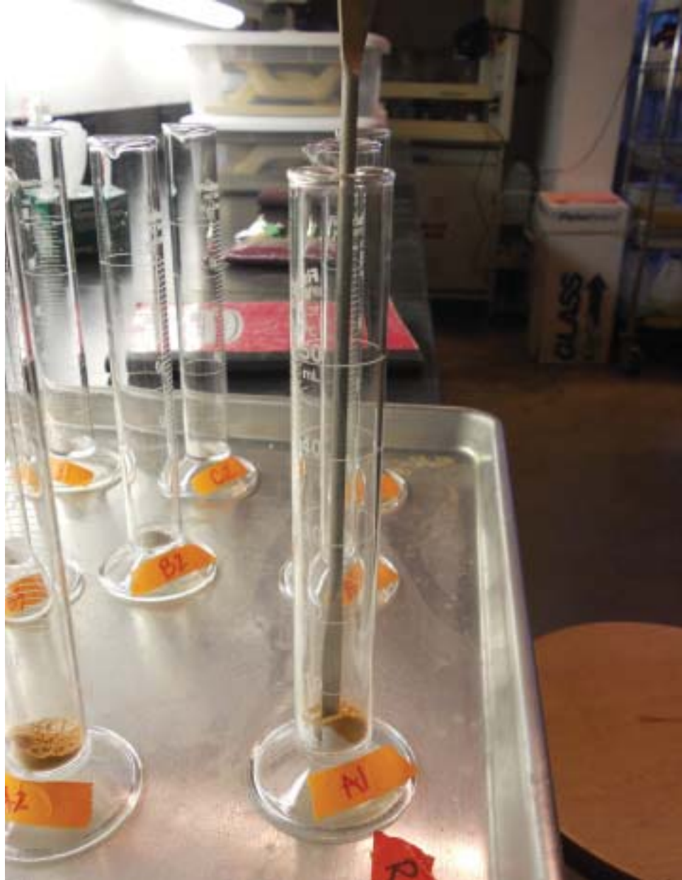
Figure 6.8: Mixing of lime and brick dust for Lime Combination Test (Rogers)
