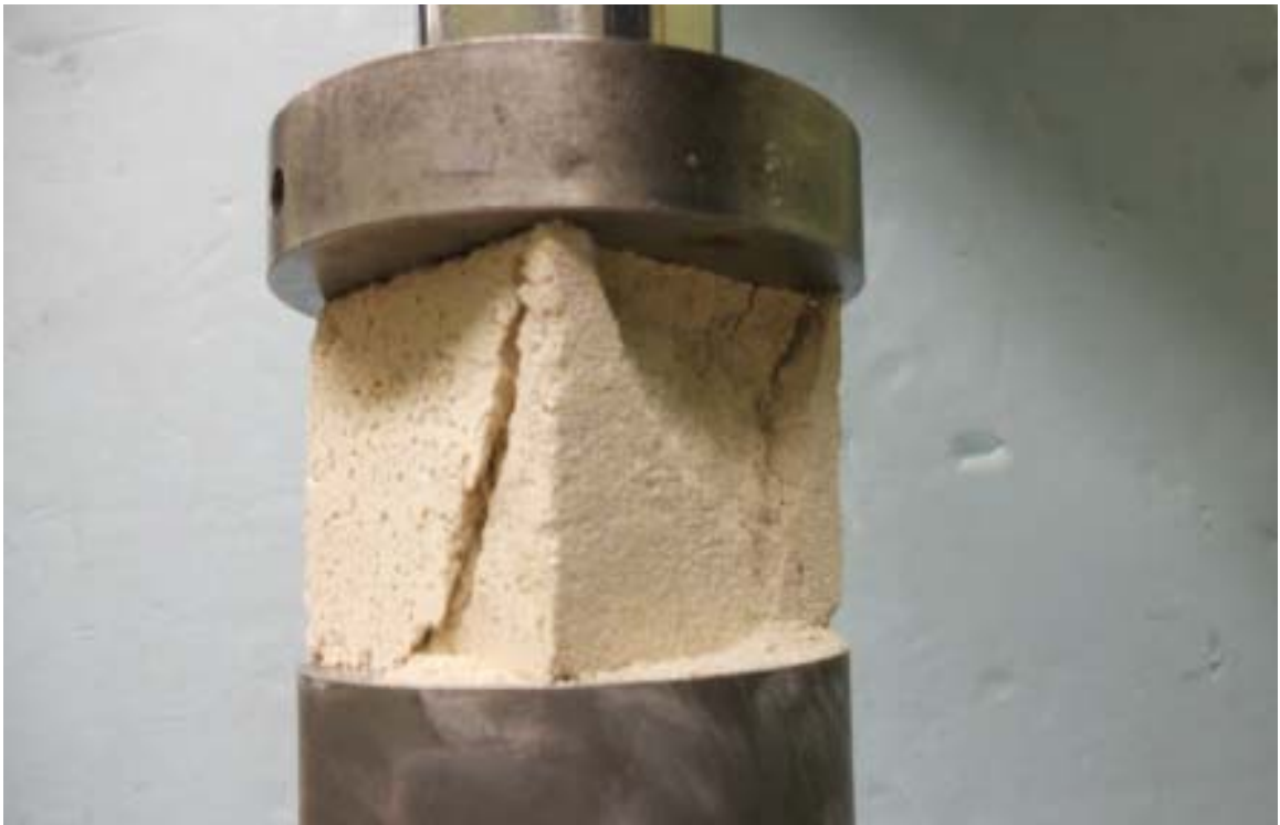
Figure 7.19: Compressive Strength Test, Formulation C mortar cube after crushing (Rogers)
