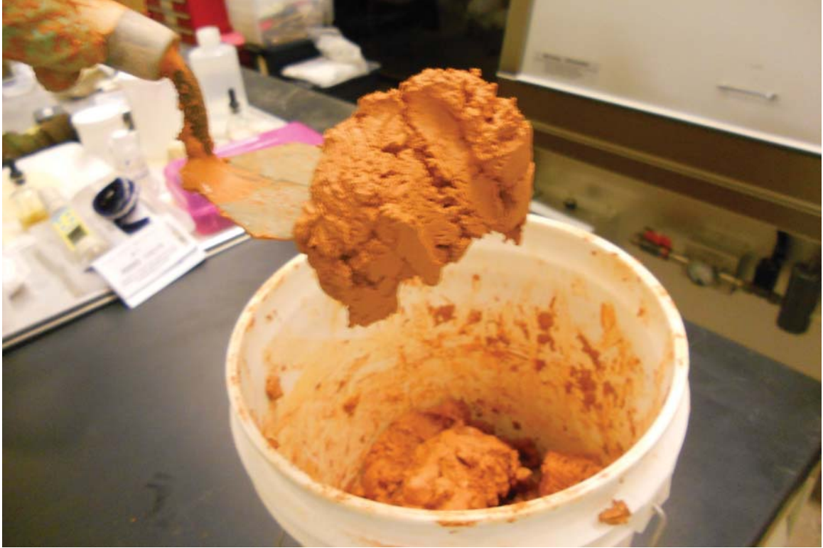
Figure 6.3: Handmixing lime and Williamsburg brick dust for underwater set test (Rogers)
