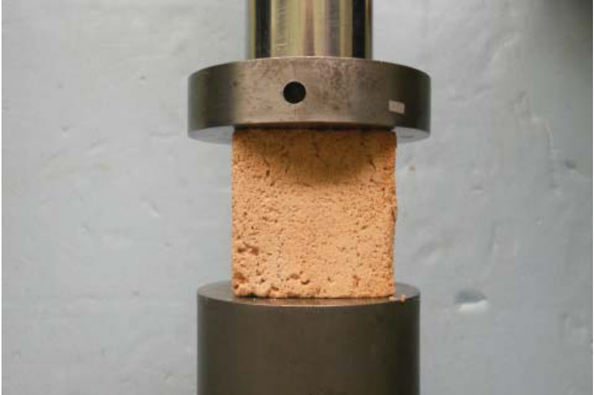
Figure 7.14: Compressive Strength Test, Formulation A mortar cube before crushing (Rogers)
