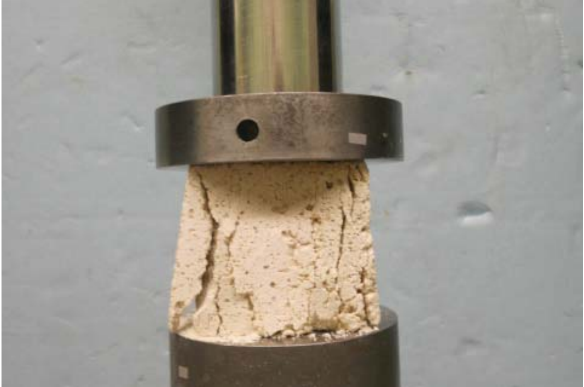
Figure 7.18: Compressive Strength Test, Formulation C mortar cube after crushing (Rogers)
