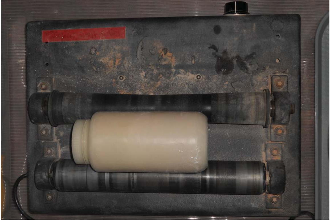
Figure 5.1: Reducing particle size of brick using ball mill (Rogers)
