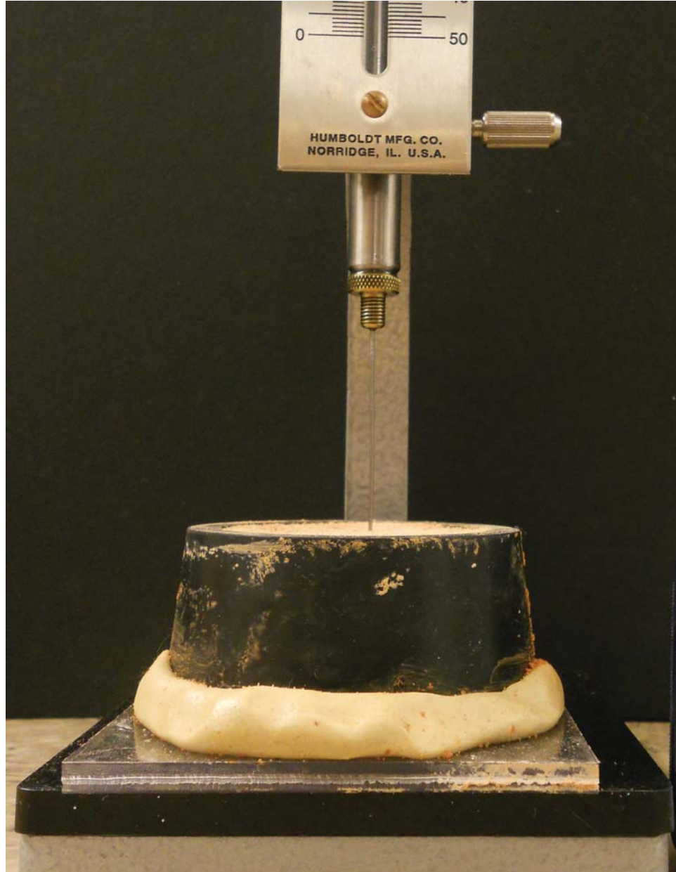
Figure 6.2: Setting time measurement using Vicat apparatus (Rogers)
