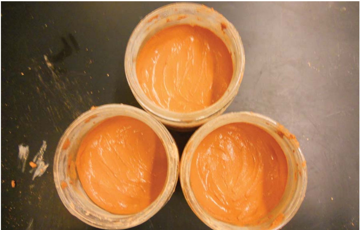
Figure 6.4: Formulation A pastes molded into glass jars before submerging in water for underwater set test (Rogers)
