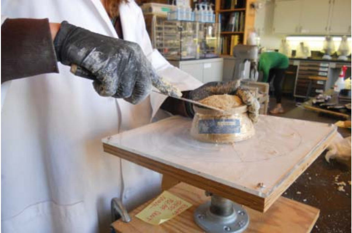
Figure 5.7: Molding Formulation B for slump test (Rogers)
