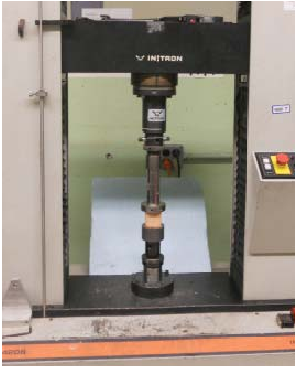
Figure 7.13: Compressive Strength Test using Instron Model 4206 at LRSM (Rogers)
