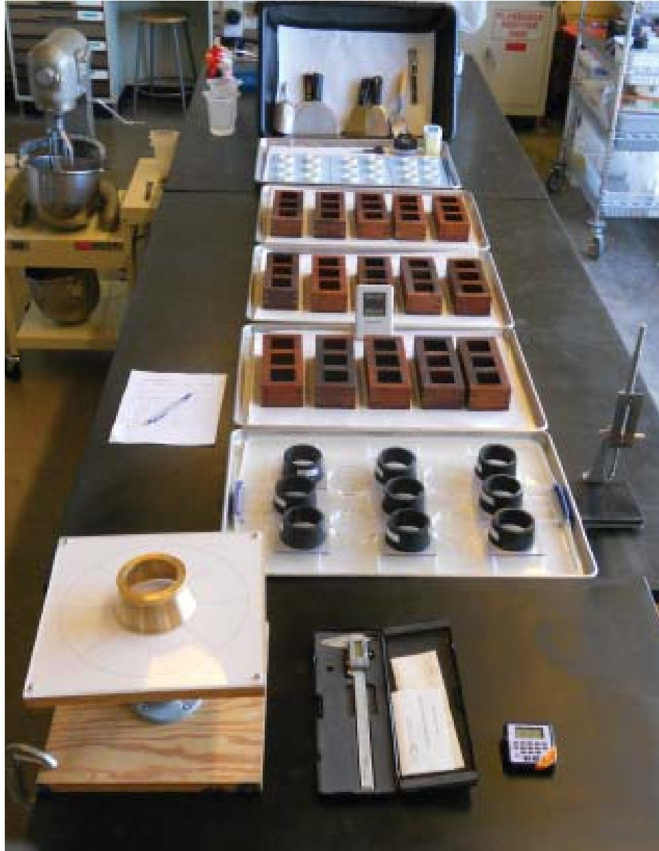
Figure 5.5: Molds and tools prepared for mixing and molding of mortar samples (Rogers)
