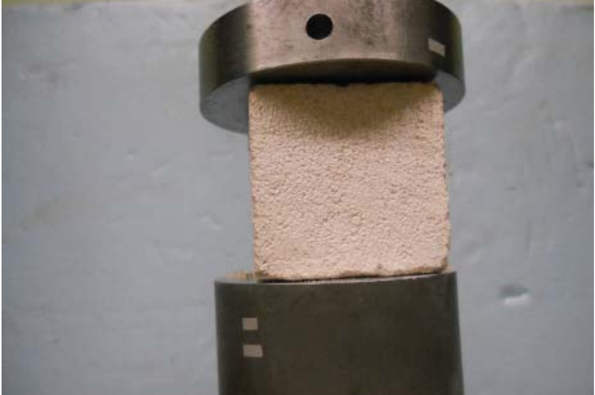
Figure 7.16: Compressive Strength Test, Formulation B mortar cube before crushing (Rogers)
