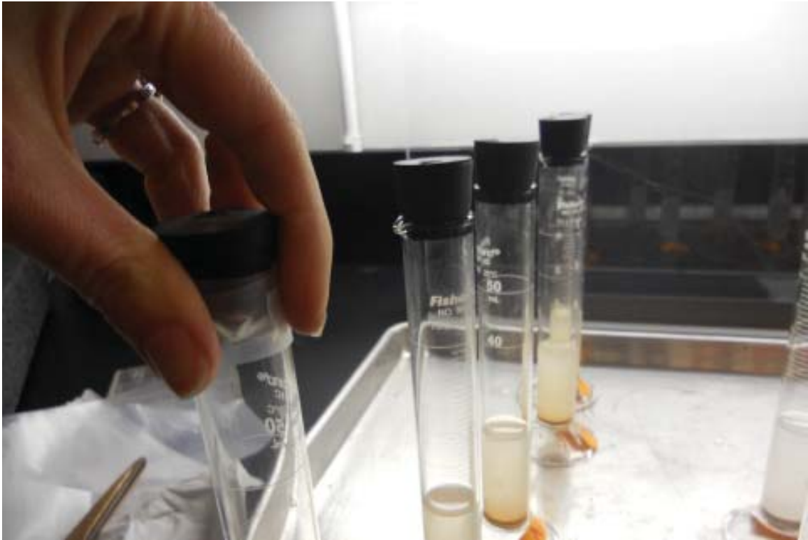
Figure 6.9: Applying Parafilm to seal cylinders (Rogers)
