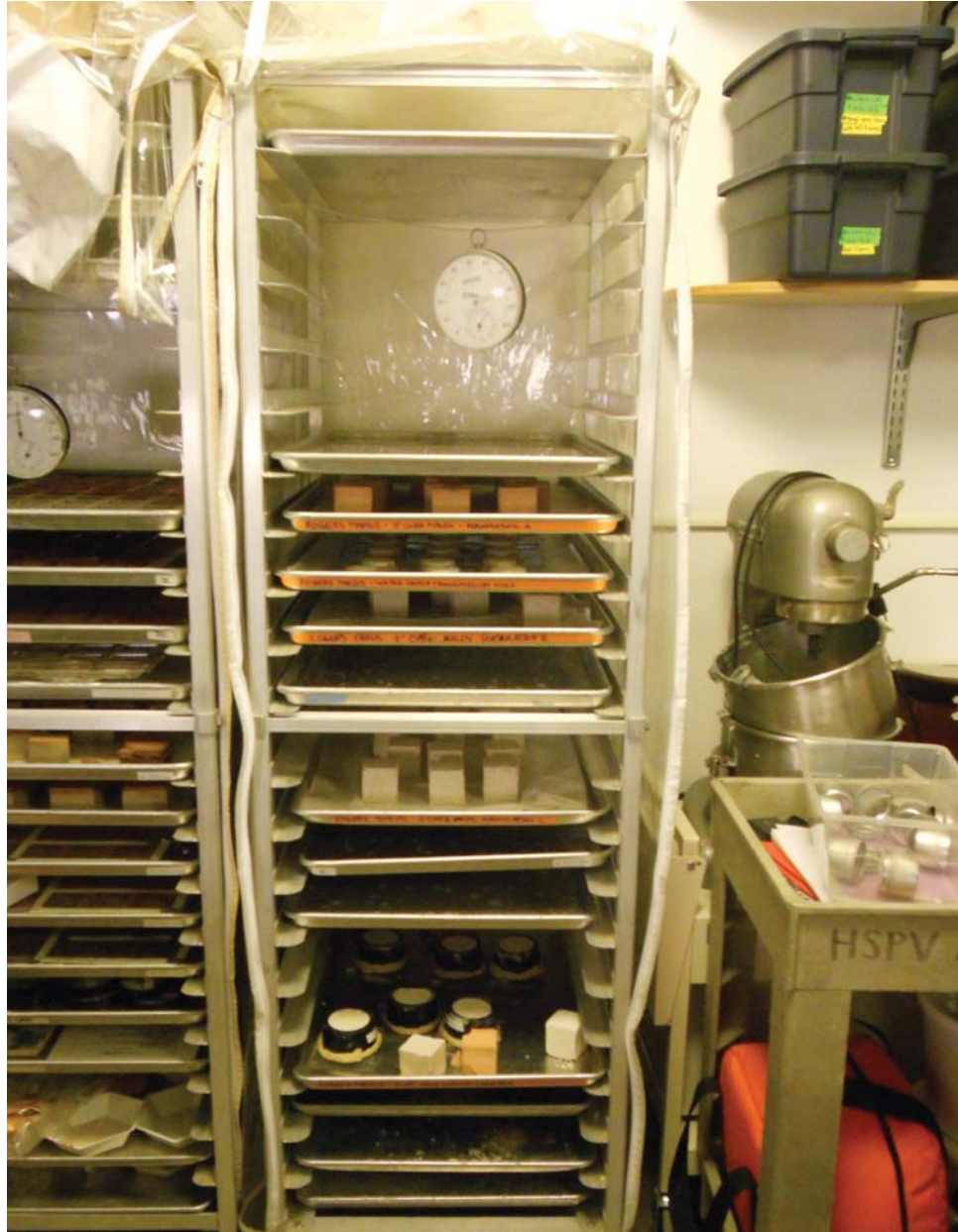
Figure 5.8: Moist cabinet for curing of mortar samples (Rogers)
