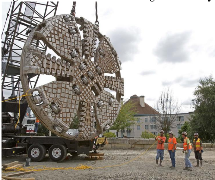
Figure 1. Cutting Head for Portland's CSO Storage Tunnel Project
