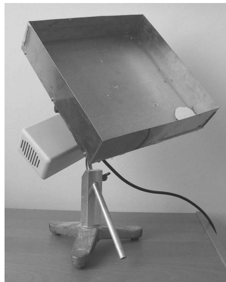
FIG. 2. The wearing apparatus used for the laboratory experiments. The rotating metal tray is 30 \times 30 \times 7 cm 3 .
