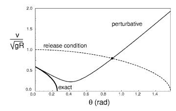
Fig. 3. Same as Fig. 2 with  $\mu$ =1. Here the first-order perturbative solution predicts that the block slows and then speeds up before reaching the release point given by the intersection with the dashed curve. The exact solution has the block slowing and coming to rest on the surface of the sphere.
