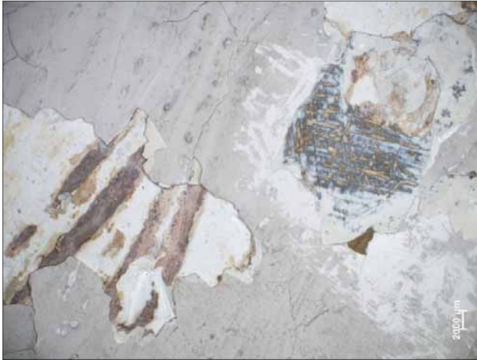
Figure 8.3. Paint exposure on fallen cornice panel, revealing mauve color in creasing, 7.1x mag, reflected light (L.Vollono, 2010).
