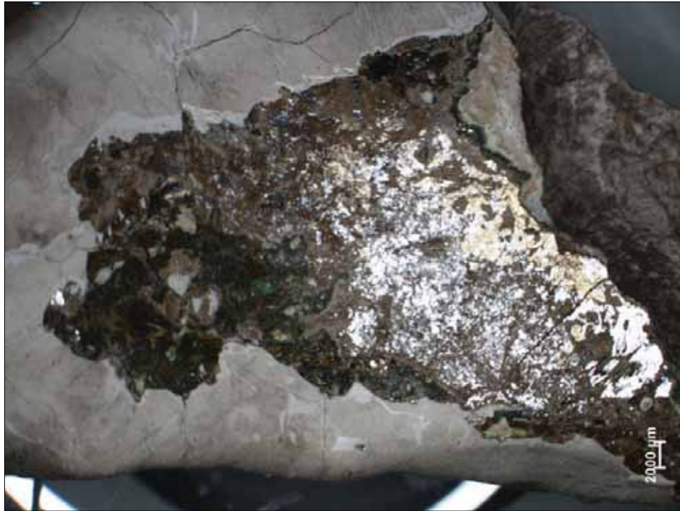
Figure 8.4. Paint exposure on fireplace flame, revealing layers of green, metallic leafing and bronzing powder, 7.1x mag, reflected light (L.Vollono, 2010).
