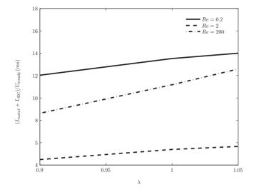
FIG. 16. Dimensional bubble residence times (milliseconds) for various Re's as a function of  $\lambda$ .
