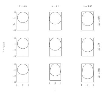
FIG. 8. Plot of steady state bubble shapes for Re=0.2, 2, and 200 and  $\lambda$ =0.9, 1.0, and 1.05.
