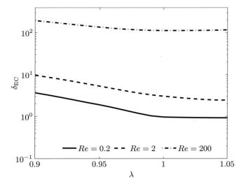
FIG. 10. Minimum film thickness normalized with  $L_{ESL}$ , as a function of  $\lambda$  for various Re's.
