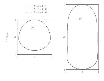
FIG. 5. Steady state bubble shapes for Re=200 and (a)  $\lambda$ =0.9, and (b)  $\lambda$ =1.3, for three aspect ratios.  $z_{\text{front}}$  denotes the axial location of the bubble's front stagnation point.
