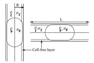
FIG. 1. Schematic of a nearly occluding bubble in vertical and horizontal vessel configurations.
