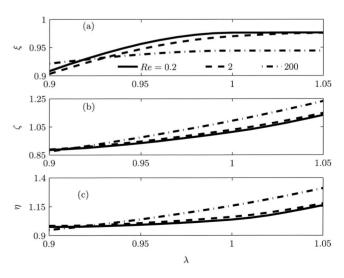
FIG. 9. Calculated bubble deformation factors for different Re's as a function of  $\lambda$ .
