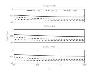
FIG. 11. Bubble steady state velocities for different Re's and  $H_D$ 's as a function of  $\lambda$ . (a)  $H_D$ =0.335, (b)  $H_D$ =0.4, and (c)  $H_D$ =0.45. Curve legends for (b) and (c) are the same as (a).
