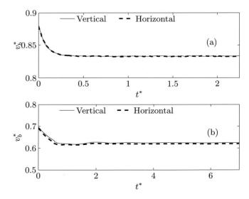
FIG. 18. Comparison of evolution of bubble velocities for horizontal and vertical vessel configurations for (a) Re=0.2,  $\lambda$ =0.9, and (b) Re=200,  $\lambda$ =0.9.
