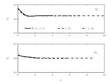
FIG. 4. Bubble velocity for Re=200 and (a)  $\lambda$ =0.9, and (b)  $\lambda$ =1.3, as a function of time for three aspect ratios (*R*:*L*).
