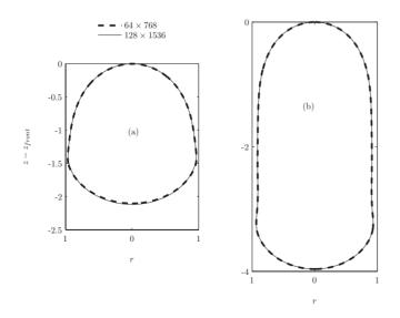
FIG. 6. Steady state bubble shapes for (a) Re=0.2,  $\lambda$ =1.0, and (b) Re=200,  $\lambda$ =1.3 with *R*:*L*=1:12 and two grid sizes 64×768, 128×1536.
