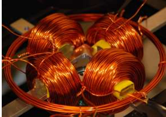
Figure 6.1: Electromagnetic coils mounted on an optical microscope to actuate the micro transporters.
