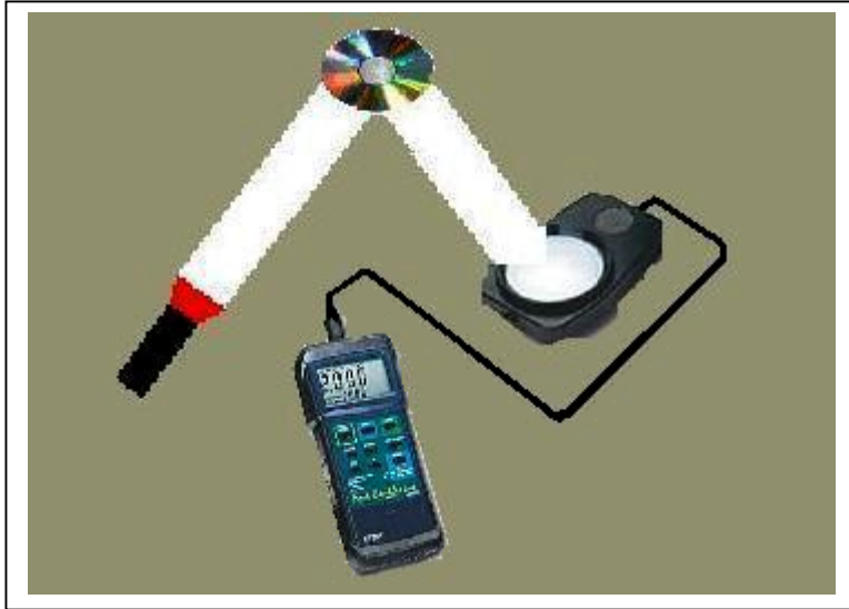
Figure 7: Testing disc reflectivity with a flashlight and a light meter. (Image by author)
