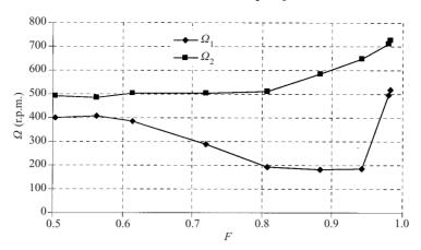
FIGURE 18. Critical conditions for the formation of bubbles in soybean oil. The experiments were carried out in a glass cylinder with an inner diameter of 1.28 cm and a length of 22.14 cm. When F < 0.4, a single air bubble is stable at any rotational speed. For  $F \ge 0.5$ , when the rotational speed is between  $\Omega_1$  and  $\Omega_2$ , separated bubbles are observed.
