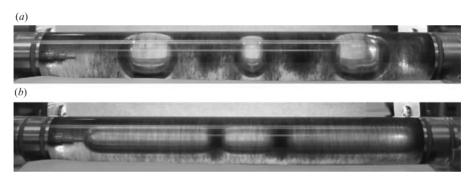
FIGURE 21. Particle segregation of resin particles with  $\rho_p = 1.13 \, \mathrm{g \, cm^{-3}}$  in glycerine with  $\rho_l = 1.173 \, \mathrm{g \, cm^{-3}}$ . The particle concentration is 8.96% and the filling level F = 0.667. (a)  $\Omega = 200 \, \mathrm{r.p.m.}$  (b) 600 r.p.m.
