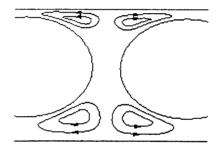
FIGURE 19. The eddies set up by the pumping motion of the off-centre bubbles. Liquid flows from the bubble to the liquid disks near the bubble surface and from the liquid disks to the bubble near the wall.
