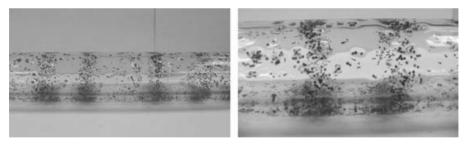
FIGURE 12. Particles which are initially distributed uniformly in a film rimming a rotating cylinder segregate into cylindrical bands (M3 in table 1). The formation of the bands takes hours.
