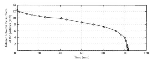
FIGURE 6. Distance between two identical nylon particles attracted by the capillary force on the glycerine–air interface.
