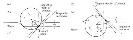
FIGURE 1. (a) Hydrophobic and (b) hydrophilic particles at equilibrium.
