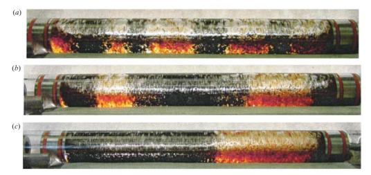
FIGURE 22. Segregation of two types of particle in a 47.8% aqueous glycerine solution with  $\rho_l = 1.09 \, \mathrm{g \, cm^{-3}}$ . The filling level F = 0.354. The concentrations of the black silicon particles and brown resin particles are 21.7% and 12%, respectively. The rotational speed is 165 r.p.m. (a) 30 min, (b) 2 h, (c) 20 h after the beginning of rotation.
