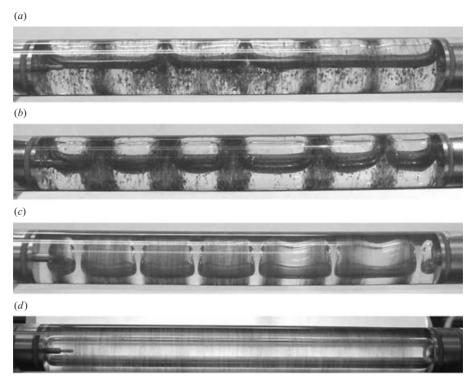
FIGURE 20. Particle segregation of resin particles with  $\rho_p = 1.13 \, \mathrm{g \, cm^{-3}}$  in the soybean oil with  $\rho_l = 0.915 \, \mathrm{g \, cm^{-3}}$ . The particle concentration is 15% and the filling level F = 0.6. (a)  $\Omega = 200 \, \mathrm{r.p.m.}$  (b) 300 r.p.m. (c) 600 r.p.m. (d) 1000 r.p.m.
