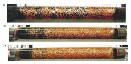
FIGURE 23. Segregation of two types of particle in a 48.7% aqueous glycerine solution. The filling level F = 0.328. The concentrations of the black silicon particles and brown resin particles are both 16%. The rotational speed is 160 r.p.m. (a) 4 min, (b) 24 min, (c) 36 min after the beginning of rotation.
