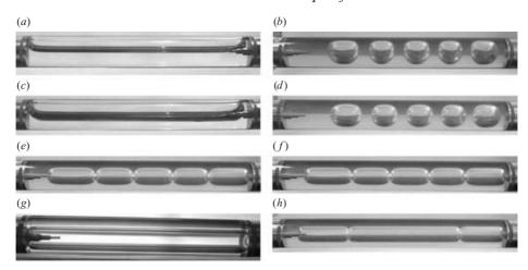
FIGURE 17. Comparison of bubble formation in (a, c, e, g) soybean oil and (b, d, f, h) Triton mixture (2950 cP). (a, b)  $\Omega = 200$  r.p.m. (c, d) 300 r.p.m. (e, f) 600 r.p.m. (g, h) 900 r.p.m.
