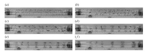
FIGURE 11. Stages of particle band formation. The experiment was performed in a low-viscosity Triton mixture at a relatively high rotational speed with a low filling level (M10 in table 1). (a) Initial distribution. (b) Particle clusters. (c) Particle blocks. (d) Initial bands. (e) Developing bands. (f) Final bands.
