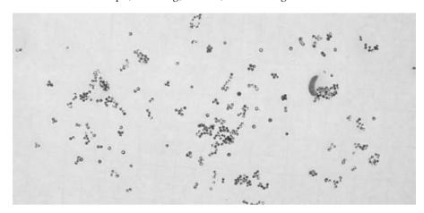
FIGURE 7. Aggregates of polymer particles in glycerine drops hanging from the bottom of a glass plate.
