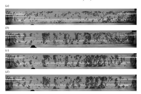
FIGURE 13. Band formation of particles due to capillarity. The liquid is water (18°C) and the particles are polymer particles. The filling level F is 0.041 and the particle concentration is 20.7%. The rotational speed  $\Omega = 8.57$  r.p.m.,  $\beta = 15.94$ , average film thickness  $D_a = 0.288$  mm, minimum film thickness  $D_{min} = 0.0213$  mm,  $D_{min}/d_p = 0.033$ . (a) 3 min, (b) 1.5 h, (c) 6 h, (d) 18 h after the beginning of rotation.
