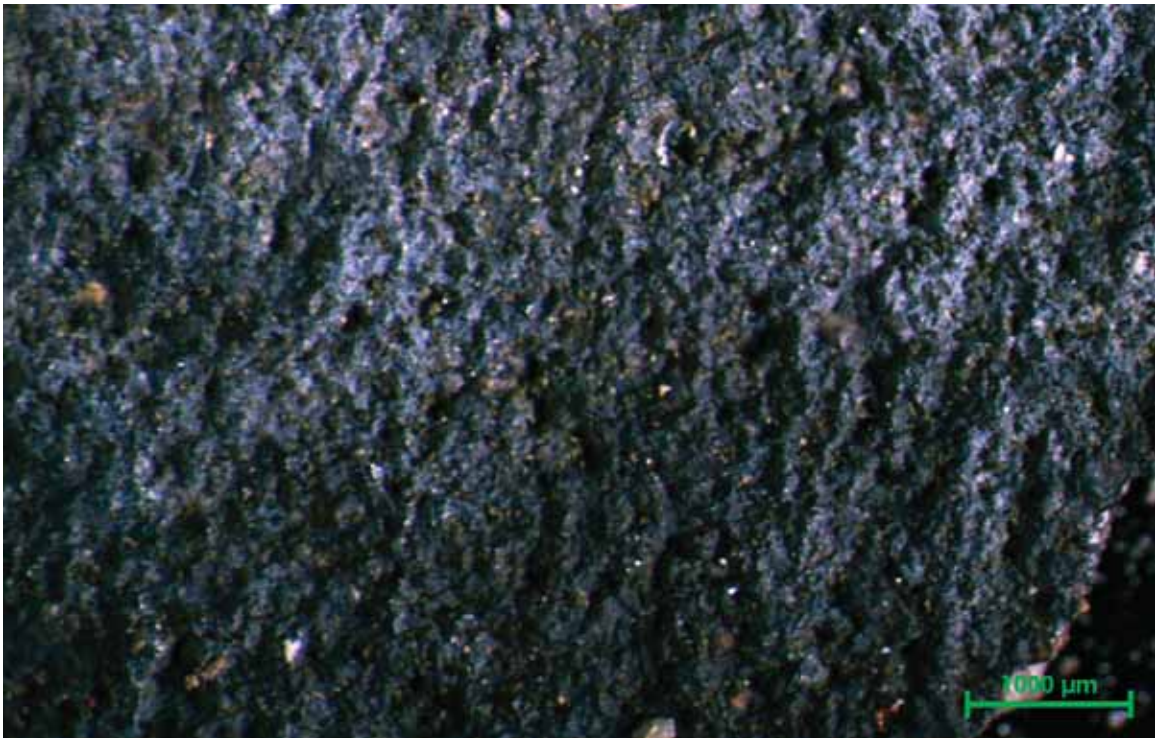
Figure 6.25 Surface detail of opaque peeling, 50x, Leica MZ16 stereomicroscope, reflected light (Source: E. Kemery, 2009)
