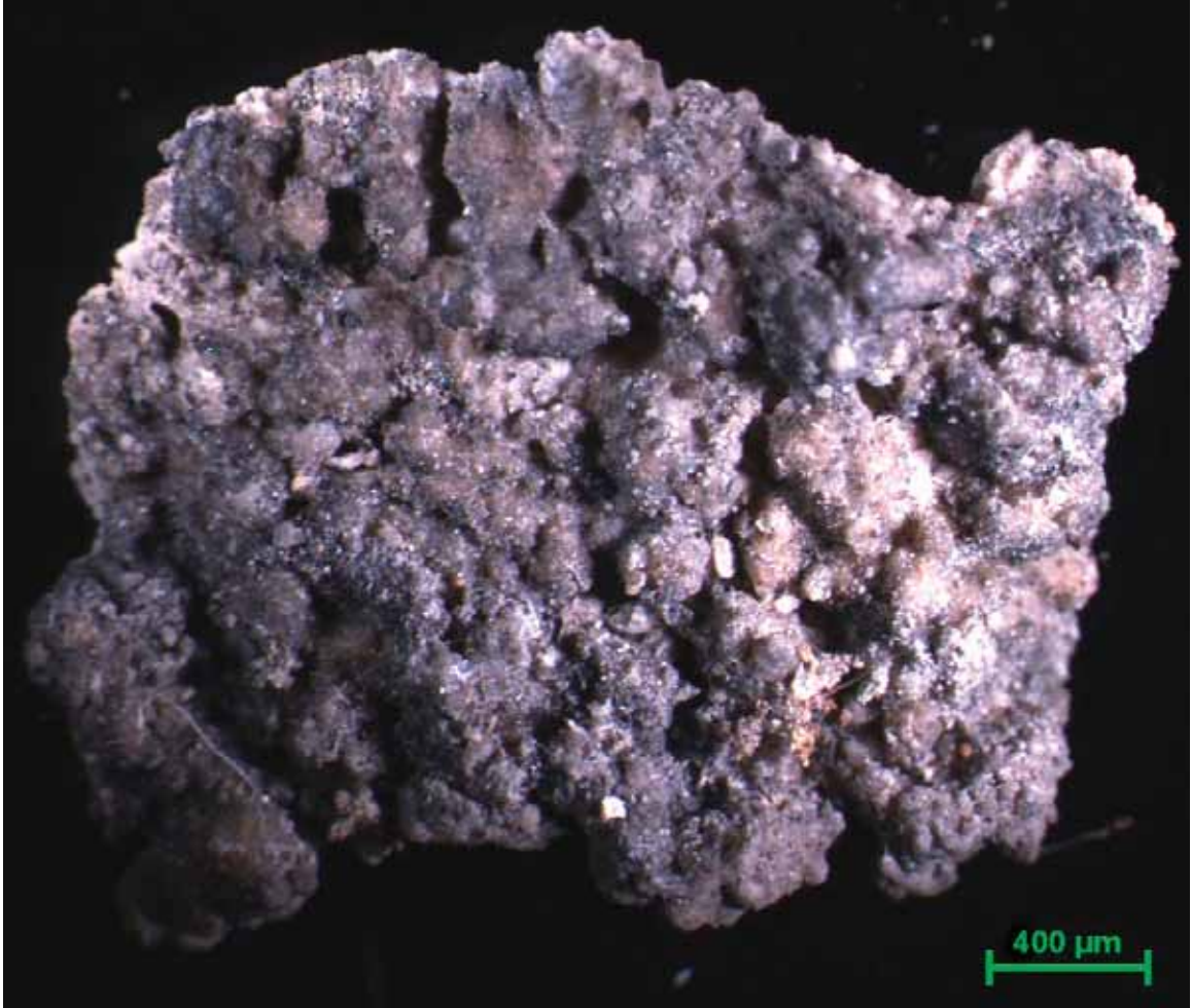
Figure 6.29 Sample of blistering, 20x, Leica MZ16 stereomicroscope, reflected light (Source: E. Kemery, 2009)
