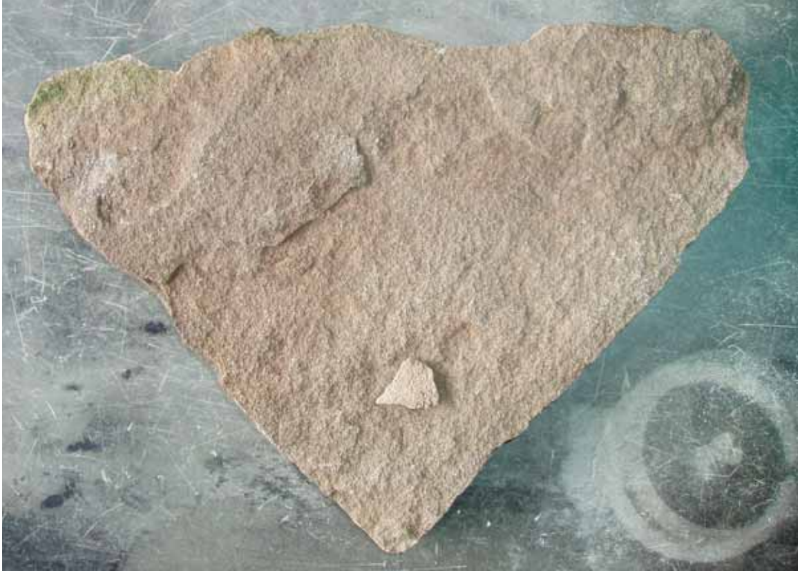
Figure 7.10 Stone sample and original mortar sample from a narrow joint (Source: E. Kemery, 2009)
