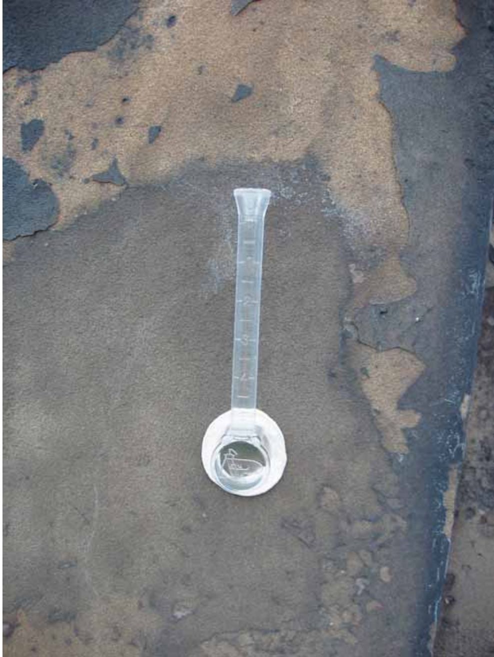
Figure 4.11 RILEM tube testing in situ on a case-hardened surface (Source: E. Kemery, 2009)
