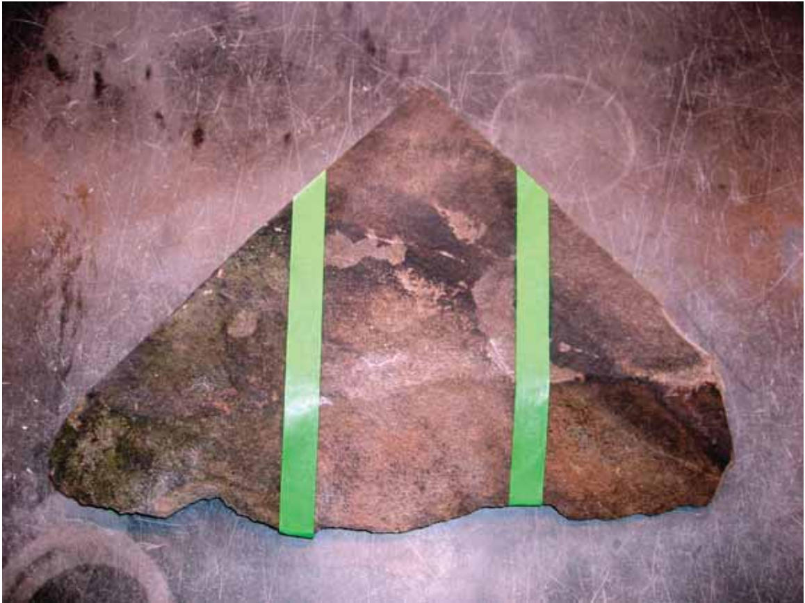
Figure 7.1 Pilot cleaning tests with PROSOCO, Inc. Sure Klean® Heavy Duty Restoration Cleaner; control (left), 1:3 cleaner to water solution (middle), 1:6 cleaner to water solution (right) (Source: E. Kemery, 2009)
