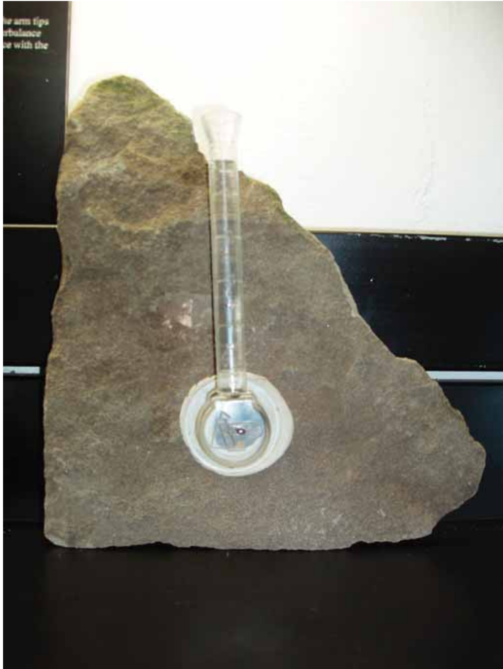
Figure 4.12 RILEM tube testing in the lab on sandstone control sample (Source: E. Kemery, 2009)
