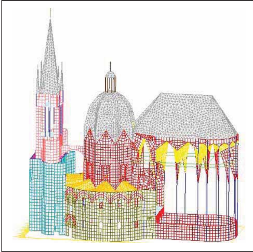
Figure 26. The complete mesh of the Aachen Cathedral, Germany. From Mistler et al. , 2006.
