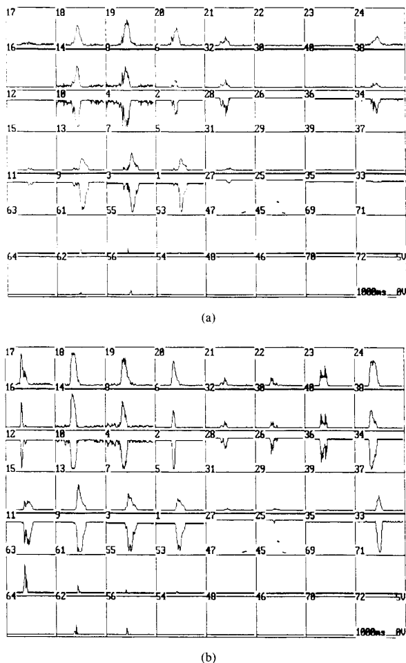
Fig. 12. Output voltages of 56 neurons during a 1000-ms time slice from a network configured for acoustical pattern analysis: (a) pattern for an "ah" sound, and (b) for a "dah" sound. Horizontal: 1000 ms; vertical: 5 V.
