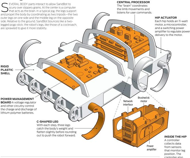
side moving in sync with the middle leg on the opposite side. The two tripods alternate supporting and propelling the body, then circle around after each step.
