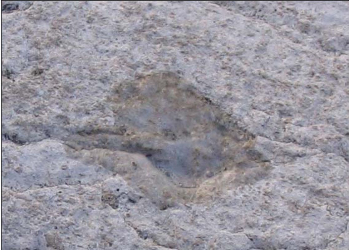
Figure 4.8: Detail of hydrochloric acid effervescing on Dayton limestone indicating the presence of calcium carbonate.
