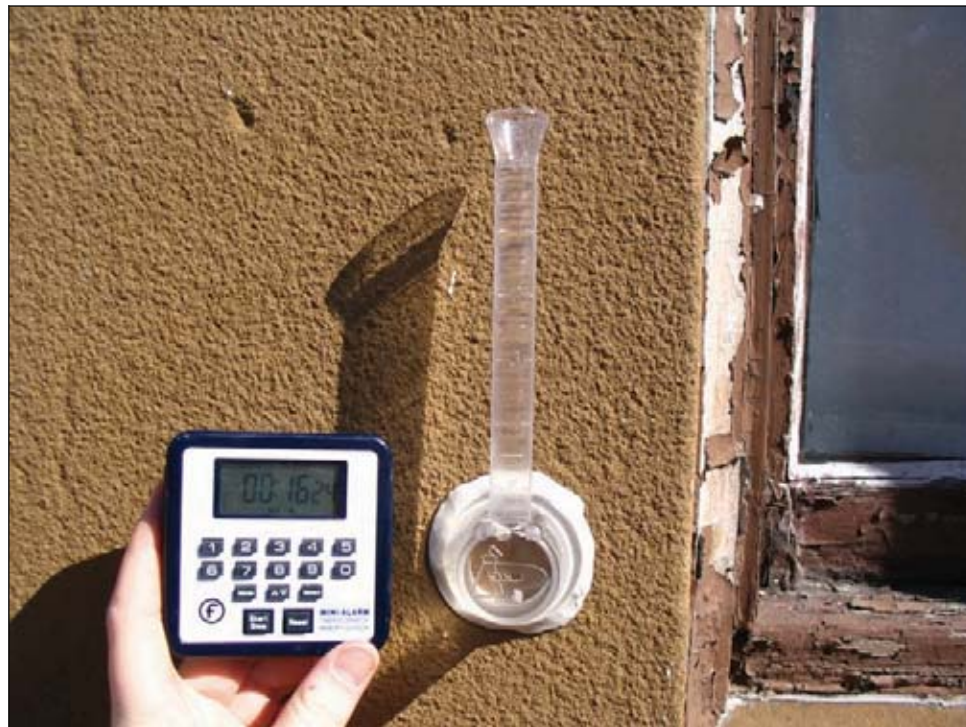
Figure 4.6: Rilem Water Absorption Test on Columbus Sandstone ( W. Fish & Co. ), note zero water absorption after 16 minutes.
