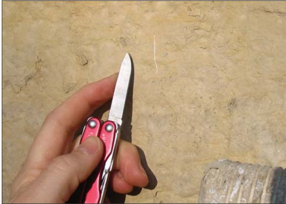
Figure 4.7: Mohs hardness test indicating Springfield limestone is softer than 5.5.
