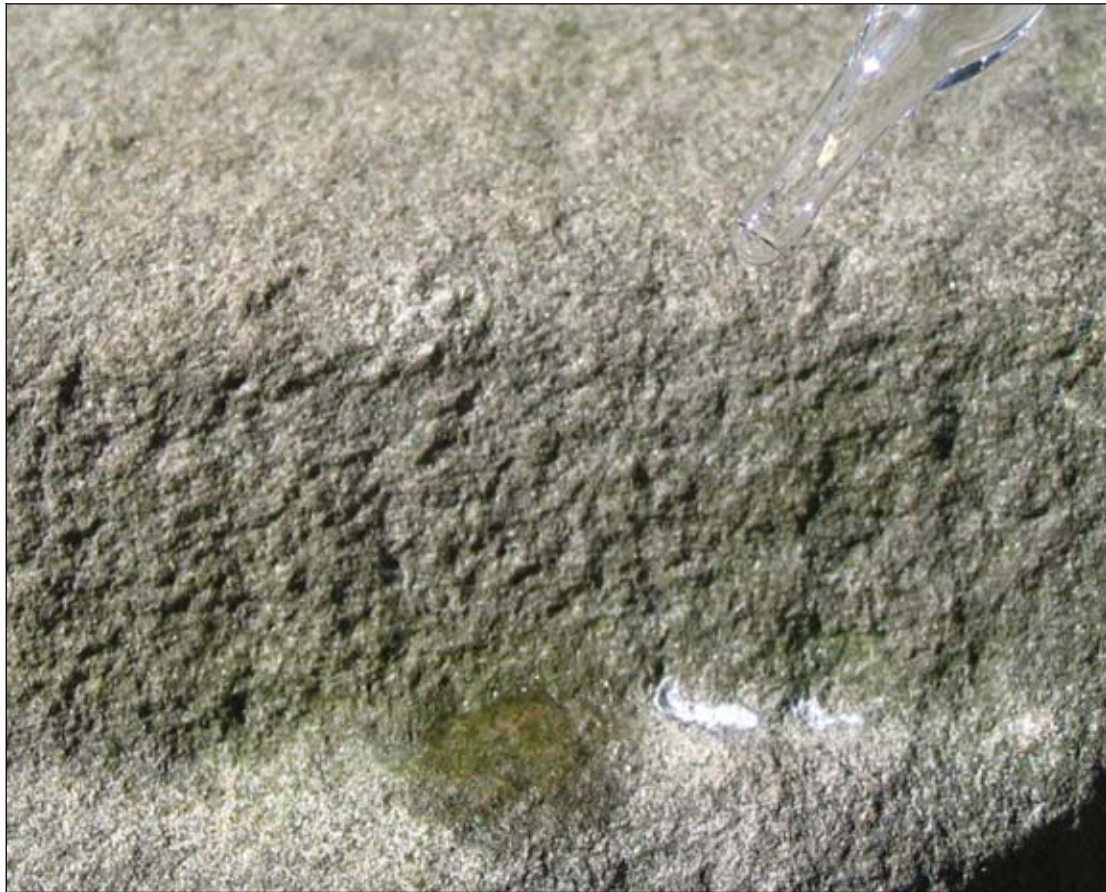
Figure 4.9: Detail of hydrochloric acid not effervescing on Berea sandstone.
