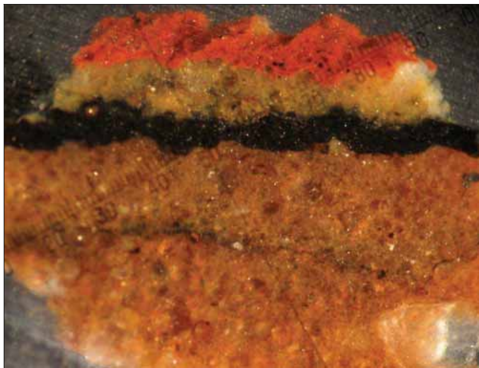
Figure 6.1. Photomicrograph of sample M07 exhibiting a fragment of bright red wash from the mid-face of Pilaster 1. Viewed in reflected light at 50x magnification.
