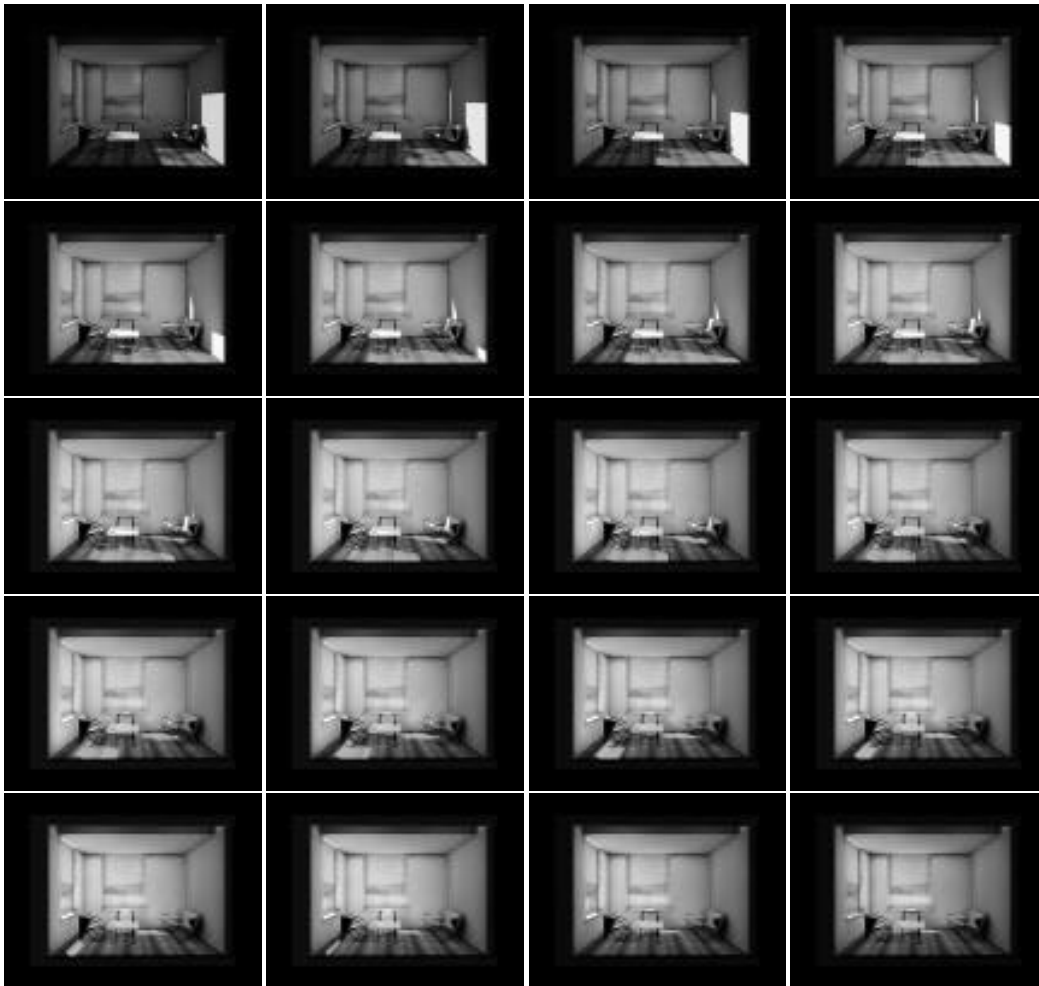
Fig. 11. Sun from 7:00am through 11:45am in 15 minute increments. Each of these 20 images is computed via linear combination of the 9 basis images.
