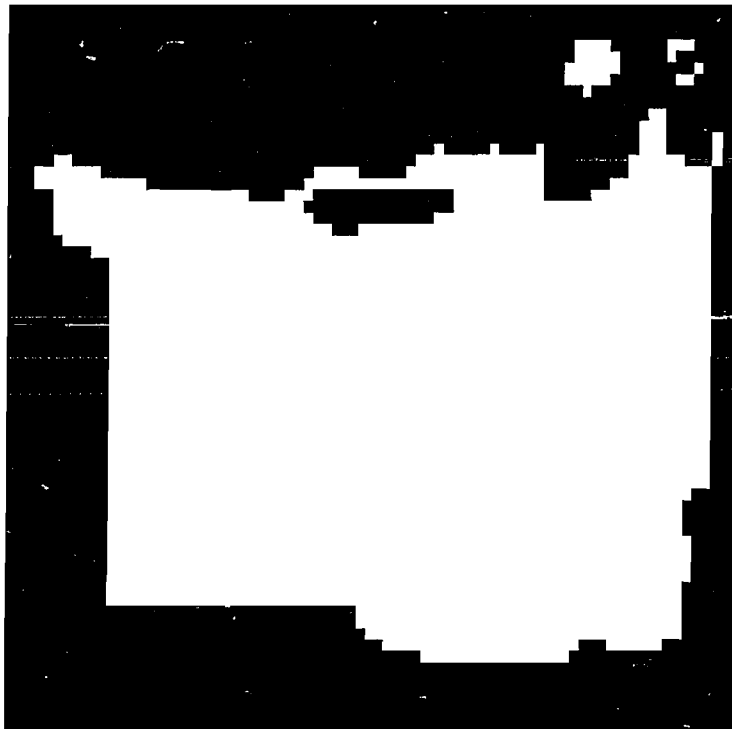
Figure 22: Segmentation into stationary and moving regions. Pixels near the edge of the image can not be classified due to the edge effects of the convolutions used to extract image flow. The segmentation correctly classifies 91.0% of the sky points and 96.9% of the ground points.
