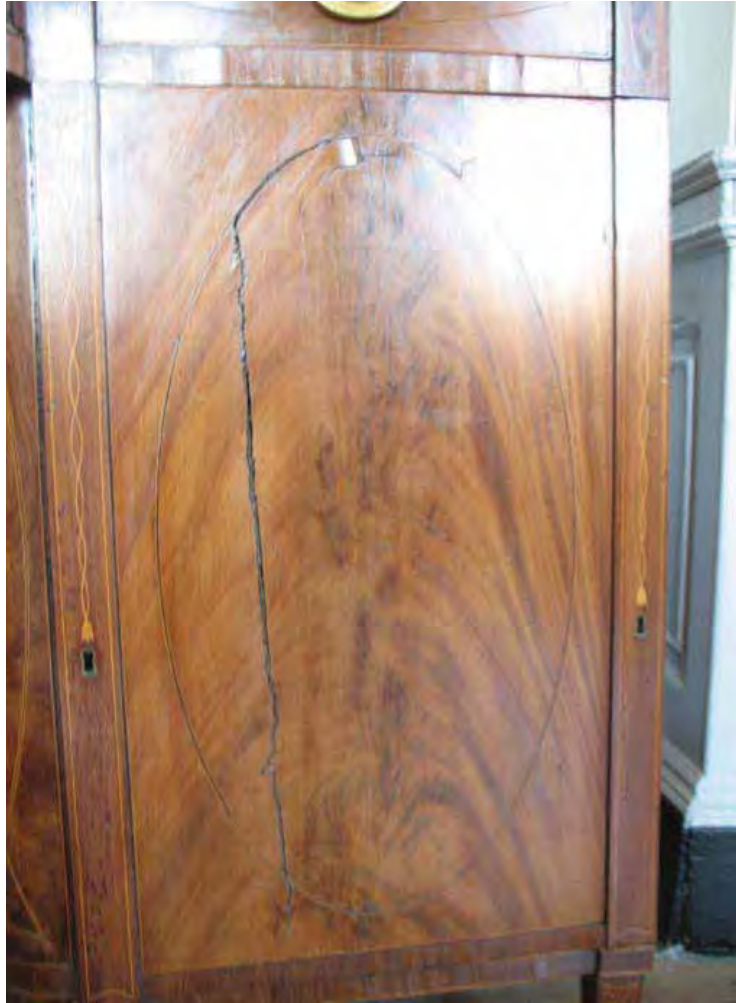
Figure 24: Federal-era Sideboard , Joseph Manigault House, photo by author, January, 2008 Note the large crack in the veneer on the cabinet door
