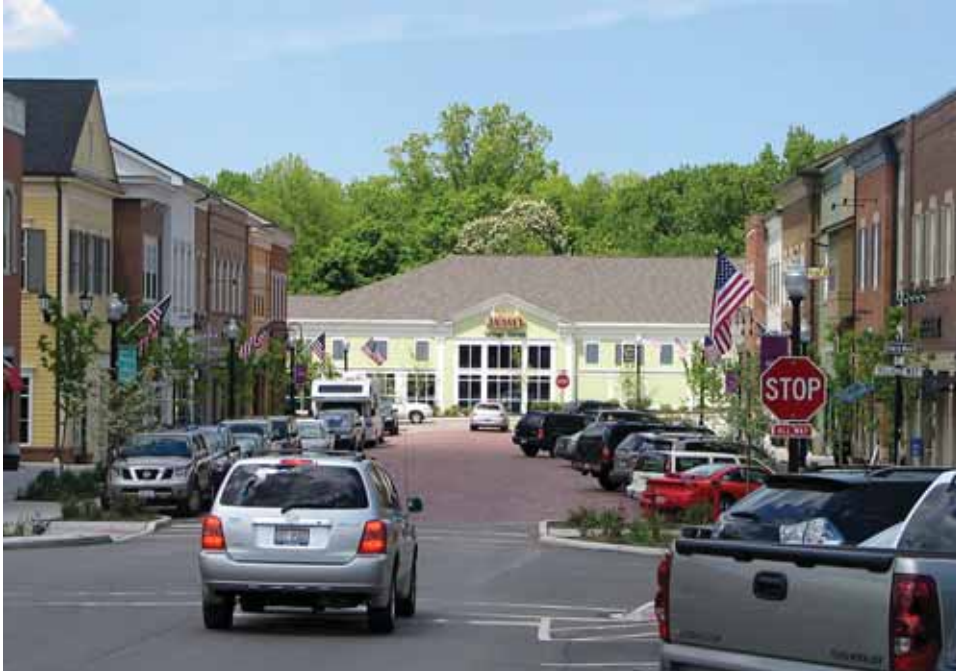
FIGURE 15. First & Main's streets are too wide relative to the height of the new buildings, which in addition to a large amount of surface parking creates an exposed feeling that dampens the pedestrian experience. Image by Dan Burden, http://www.co.weld.co.us/compplan/presentations/Dan%20Burden%20Walkability%20June%202007_files/slide2484_image392.jpg
