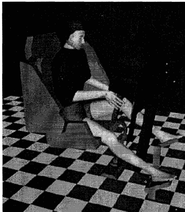
Figure 2. Smooth body Jack as virtual occupant in an Apache helicopter CAD model.
