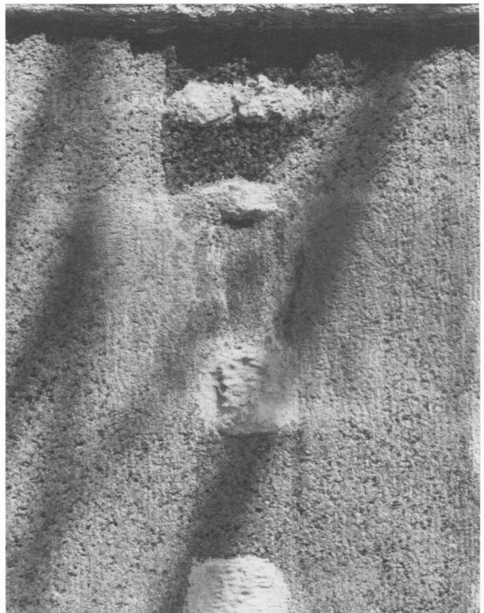
30. Comparative results of 150-psi cleaning with all four aggregates.
