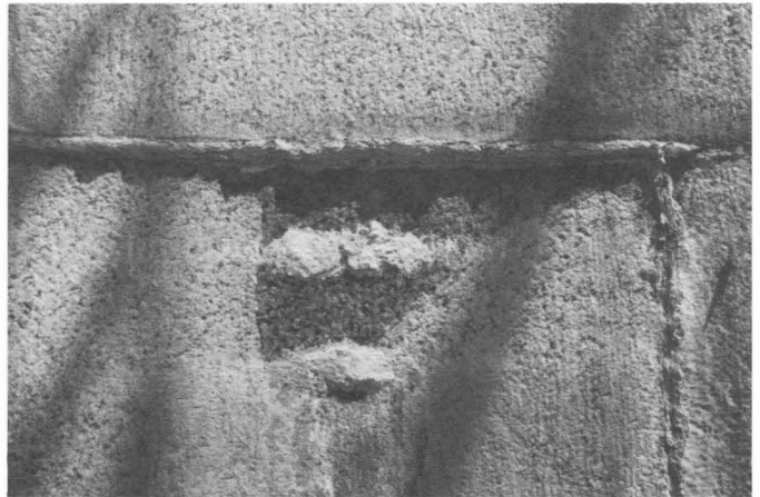
28. Area after 150-psi cleaning with flint shot sand (A3) and slag (B3).
