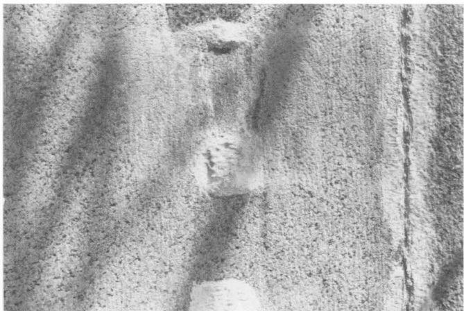
29. Area after 150-psi cleaning with walnut shells (C3) and sharp-edged sand (D3).
