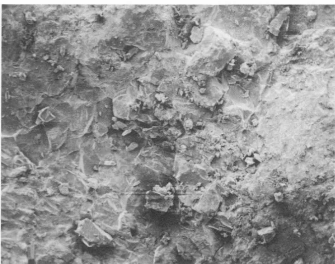
36. Scanning electron photomicrograph of granite control surface after 150-psi cleaning with slag (mag.: 50x).
