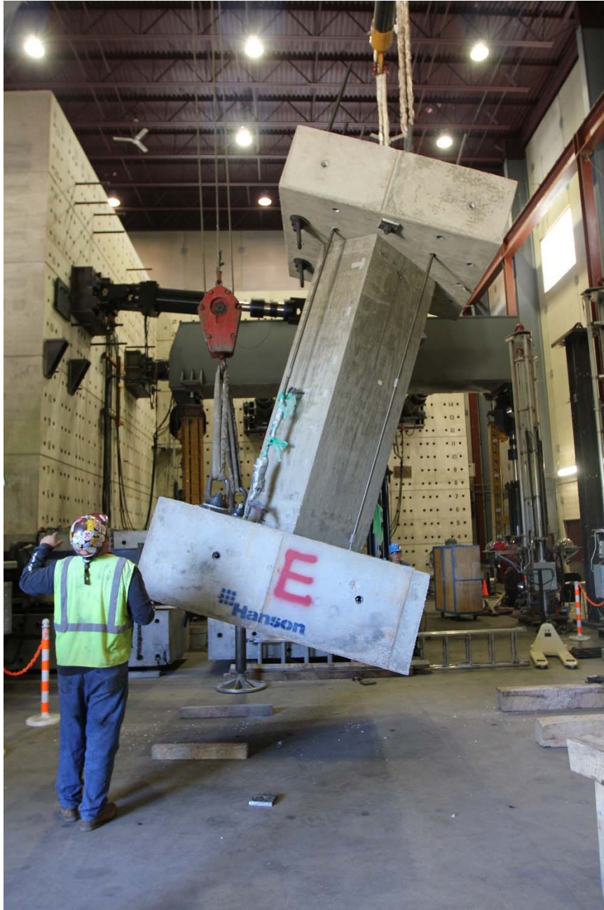
Figure A.16. Tilting Up the Specimen at the MAST Lab
