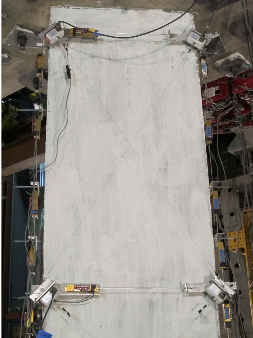
Figure A.11. Installation of LVDTs and String Pots on NE Face of the Column
