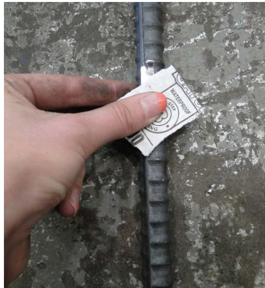
Figure A.7. Grinding and Cleaning of Bars Prior to Strain Gage Installation
