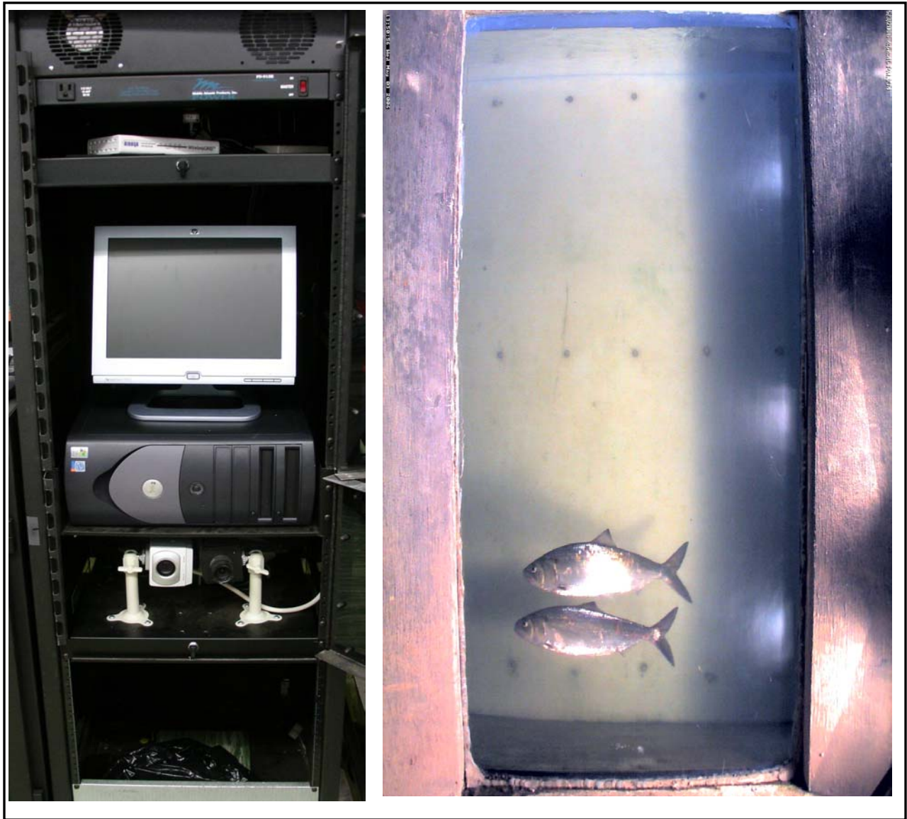
Figure 8. Picture of digital video monitoring system used in viewing room at Fairmount fishway (left) and viewing window with two American shad passing through (right).
