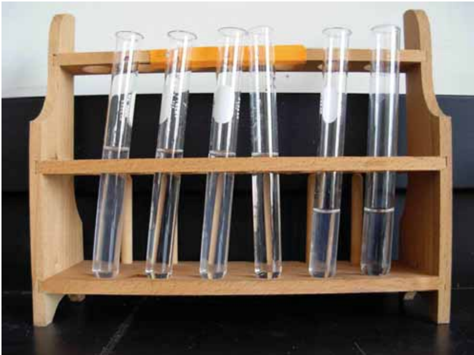
Figure 86. Photograph of the chloride salt ion laboratory test results of the water taken from the existing well on the Abel and Mary Nicholson house property. Notice the difference in clarity between the well water and the control. (Source: A. Aiken; Taken 3/22/2007.)
