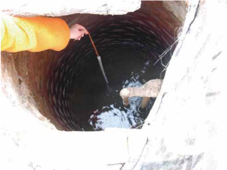
Figure 83. Photograph of bailer sampling of the existing well near the south elevation of the Abel and Mary Nicholson house. (Source: A. Aiken; Taken 3/8/2007.)
