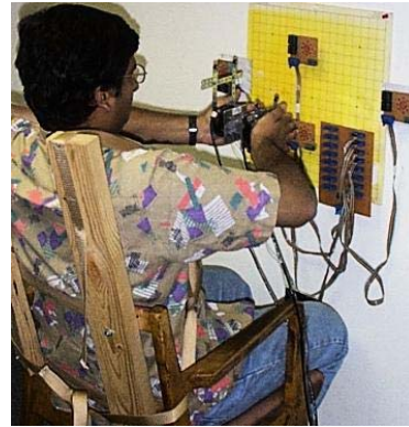
Figure 4.5: a) Force sensors with infrared markers b) Experimental system for vertical movements.
