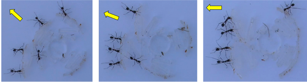
Figure 8.6: Video frames showing configurations of ants that resulted in motion of the first PDMS prototype. The yellow arrow shows the direction of movement in each frame. Note that the ants are predominantly arranged on one side of the load, in contrast to the arrangement of ants on both sides of the lighter Lexan load.
