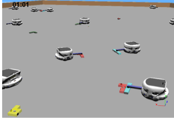
Figure 7.2: Snapshot of the arena in the realistic physical simulation. Robots carry parts at the end of a protruding bar.
