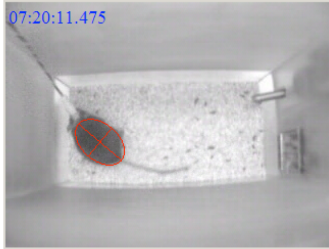
Figure 7.1: One frame of video data with an ellipse imposed by the tracking program that is used to calculate size, aspect ratio, and velocity of the mouse. Subtle differences between the three states can be detected visually suggesting some hope for the endeavor of automated sleep scoring.
