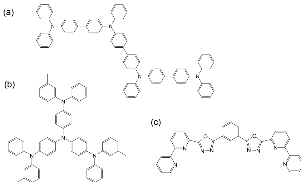
Figure 11.4 Molecular structures for TPT1 (a), m-MTDATA (b), and Bpy-OXD (c) which demonstrate varying degrees of uniaxially anisotropic optical constants.
