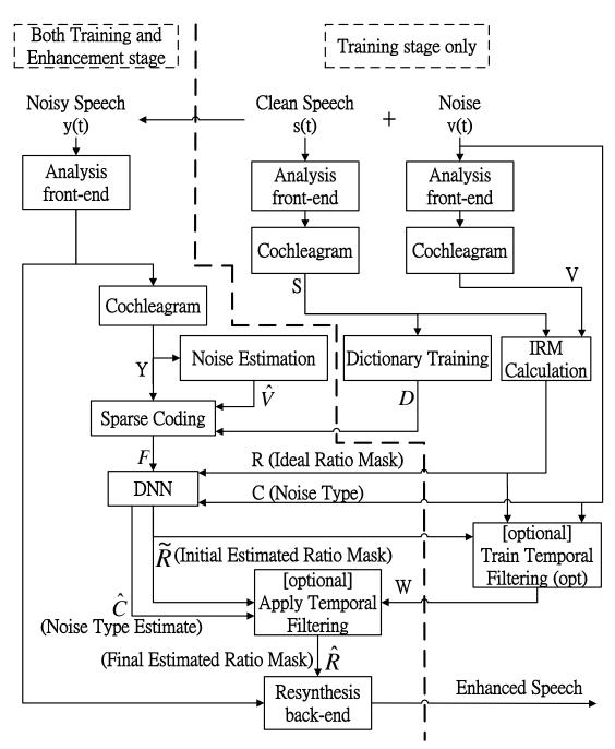
Figure 5.3: Block diagram of the proposed SNMF-DNN system. Modules on the right are those modules used only in the training stage; modules on the left are those used in both training and enhancement stage.
