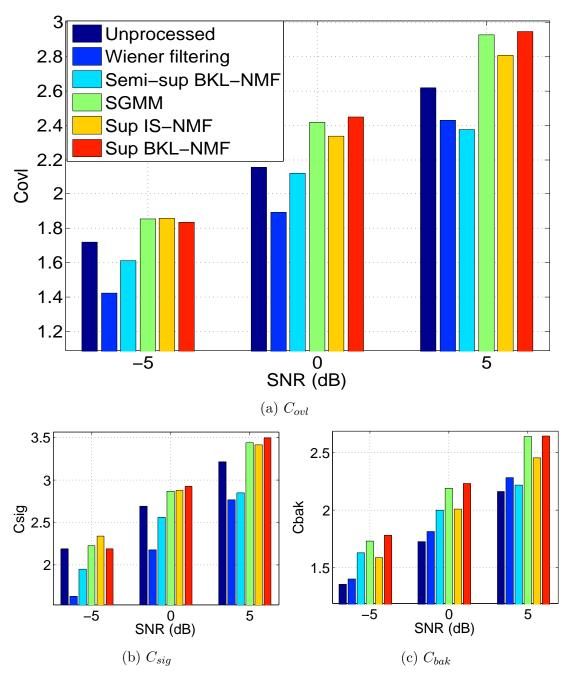
Figure 4.1: Enhanced speech quality comparison between algorithms using three objective metrics. All values are averaged across 192 randomly selected sentences and across 5 different noise types, namely, babble, factory 1, factory 2, street, and tank.
