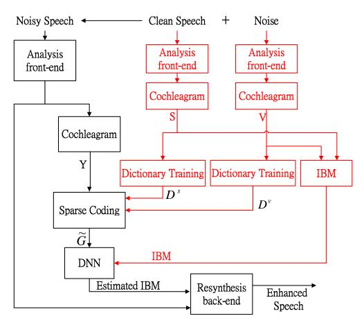
Figure 5.1: Block diagram of the SNMF-DNN-Binary algorithm. Modules highlighted in red are those modules used only in the training stage; modules in black are those used in both training and testing stage.
