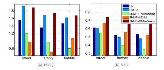
Figure 5.2: Performance comparison of the enhanced speech at -5 dB SNR under street, factory, and babble noises. "UN" denotes the unprocessed noisy mixture. "LSTSA" denotes using LSTSA [3] with MMSE noise variance tracking [4]. SNMF+Thresholding and SNMF+LSVM denotes the system that uses the same structure as the proposed system, but changes the classifiers from DNN to thresholding and LSVM, respectively. All values are averaged over 300 randomly selected sentences from the "test" data set.
