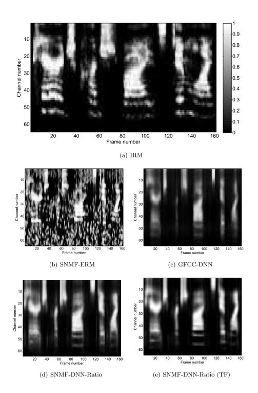
Figure 5.5: Masks estimated by different algorithms under -5 dB factory noise. The top panel denotes the ideal ratio mask, while the remaining panels shows the estimated mask by different algorithms.
