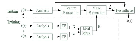
Figure 1.4: Block diagram of the general system design of IM-based approach.
