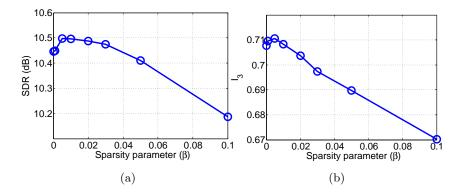
Figure 3.8: Performance of non-causal WNMF under 0 dB AWGN with different sparsity parameter  $\beta$  in the dictionary training stage. M is fixed to 480, and  $\lambda$  is fixed to 0.01.
