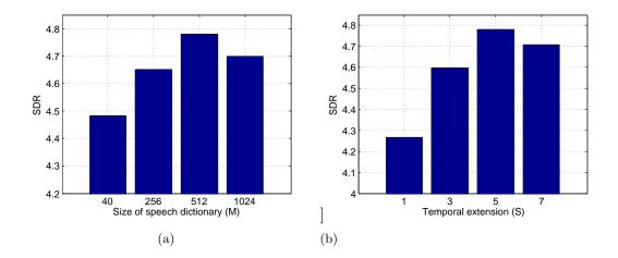
Figure 5.6: SDR of SNMF-DNN-Ratio with different size of speech dictionary and different length of temporal extension under matched training-enhancement setup (-5 dB Factory noise).
