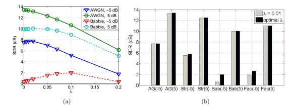
Figure 3.6: Performance under different noisy conditions with different  $\lambda$ . Fig. 3.6(a) shows the SDR change with respect to  $\lambda$ . Fig. 3.6(b) compares the SDR when  $\lambda$  is fixed to 0.01 or when  $\lambda$  is optimally chosen for each noisy condition.  $(M, \beta)$  is fixed to (480, 0.01).
