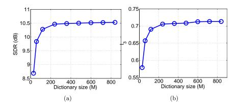
Figure 3.7: Performance of non-causal WNMF under 0 dB AWGN with different dictionary size M. Both  $\beta$  and  $\lambda$  are fixed to 0.01
