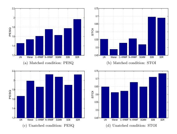
Figure 6.1: Enhancement result in both the matched and unmatched conditions. Algorithms on each figure denotes, from left to right, the unprocessed speech, the Wiener filtering, the causal WNMF, the non-causal WNMF, the SGMM, the SNMF-DNN-Binary, and the SNMF-DNN-Ratio.
