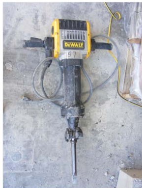
(c) Jackhammer used for chipping
