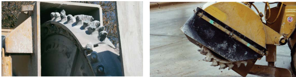
Figure 1-2 Examples of milling machines used to remove deteriorated concrete (Frentress & Harrington, Guide for Partial-Depth Repair of Concrete Pavements, 2012)
