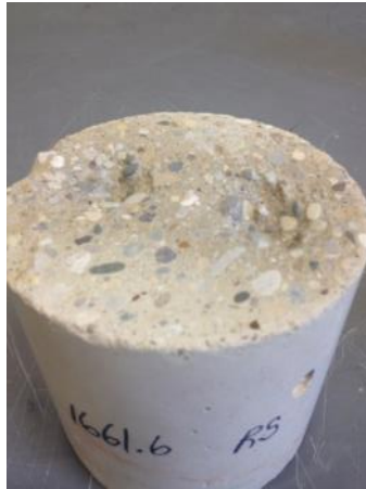
Figure 10: Abrasion resistance sample cylinder.
