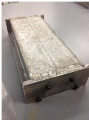
Figure 11: Length change in sulfate specimen mold.
