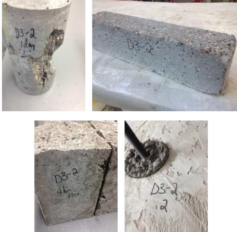
Figure 39: District 3 Mix 2 compressive, freeze-thaw, flexural and pull out specimens
