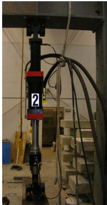
Figure 3-20 35-kip capacity hydraulic actuator, fully extended
