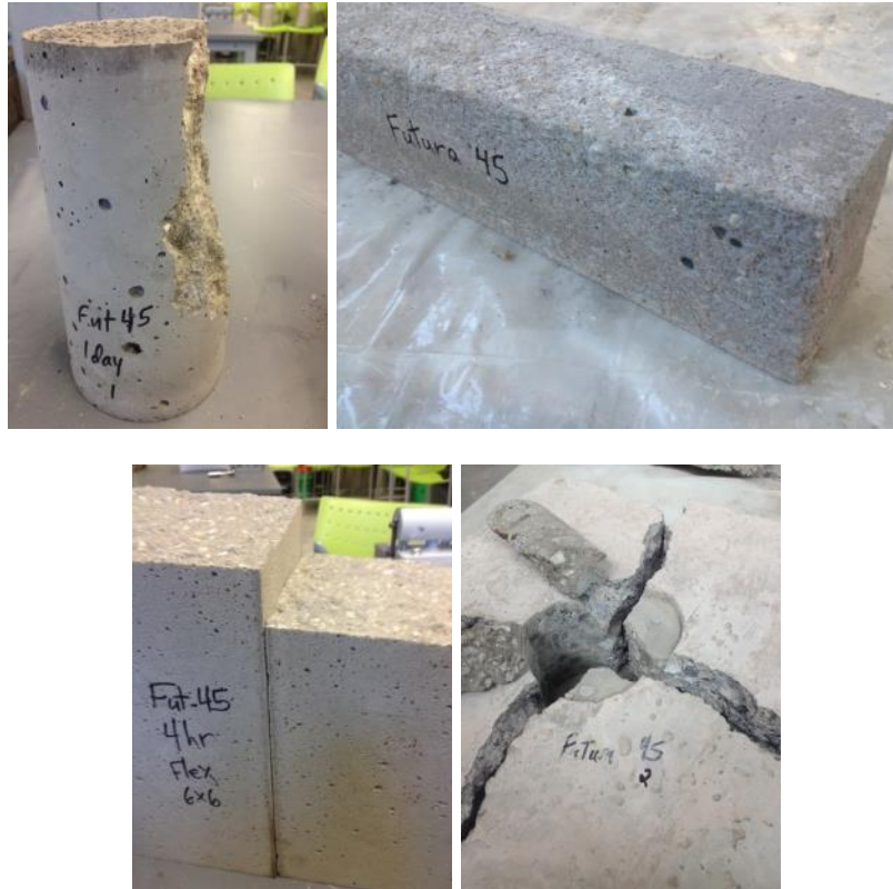
Figure 42: Futura-45 compressive, freeze-thaw, flexural and pull out specimens
