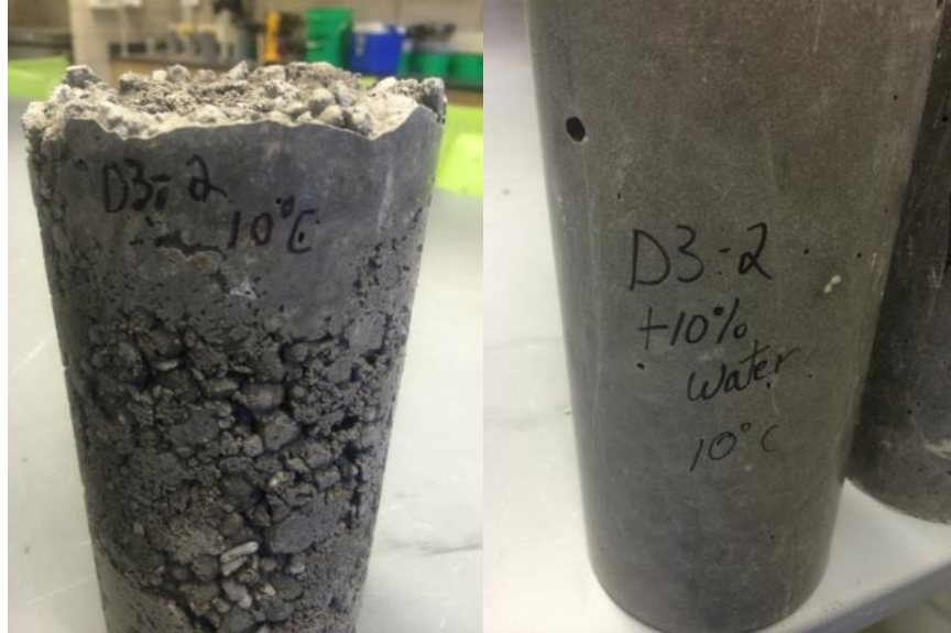
Figure 67: D3-2 mixed as per specified and mixed with 10% additional water.
