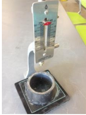
Figure 1: Vicat needle apparatus
