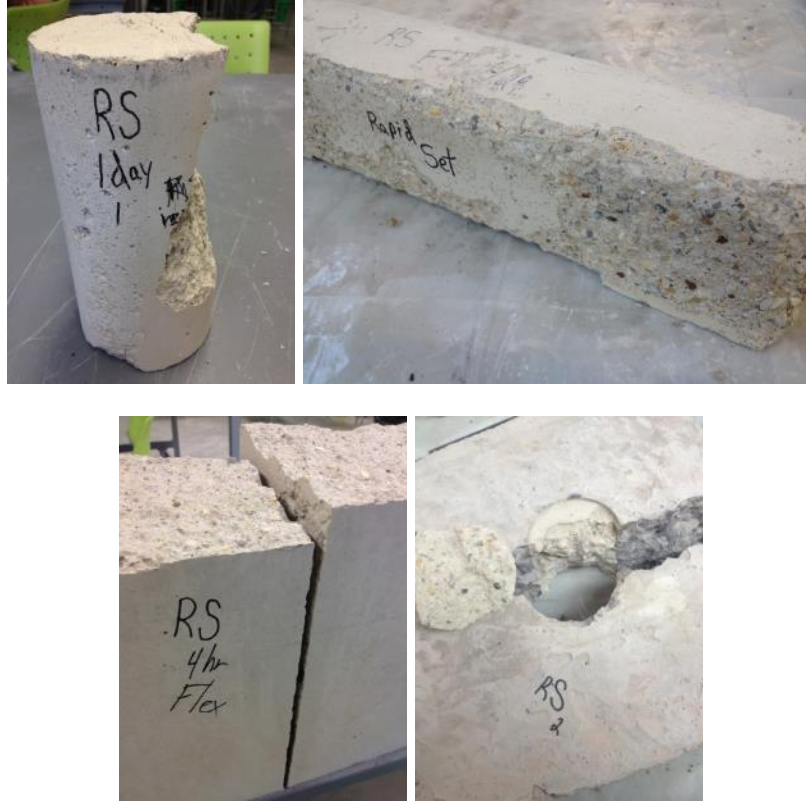
Figure 46: Rapid Set compressive, freeze-thaw, flexural and pull out specimens
