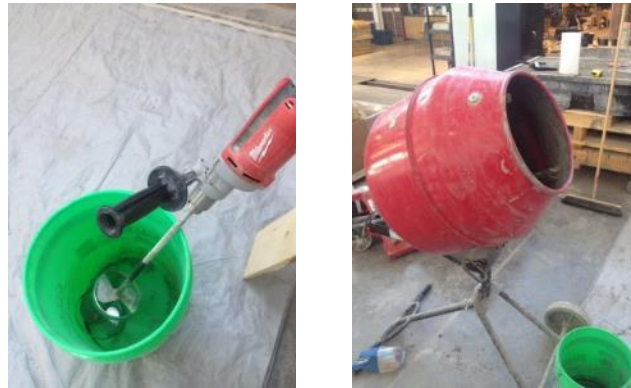
Figure 25: Drill and paddle with a bucket and a standard concrete mixer
