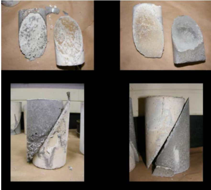
Figure 62: 3U18M on the left and Futura 45 to the right, both having slant faces intact.
