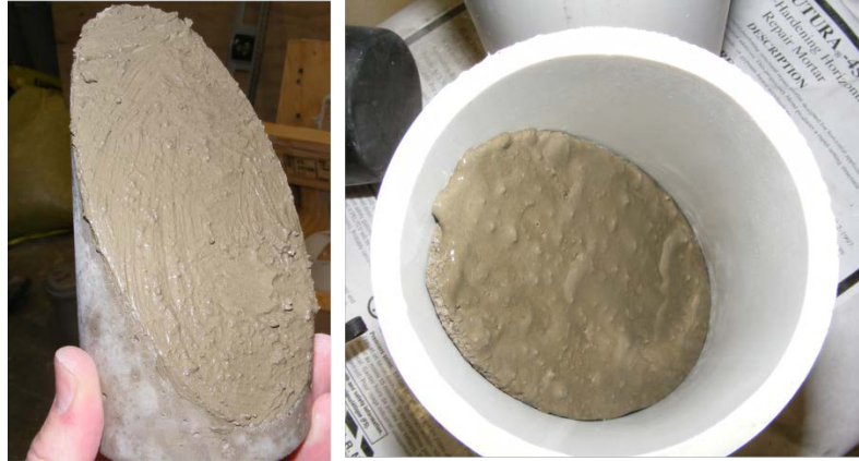
Figure 3-6 Mortar half-cylinder with cement paste applied and placed in PVC mold
