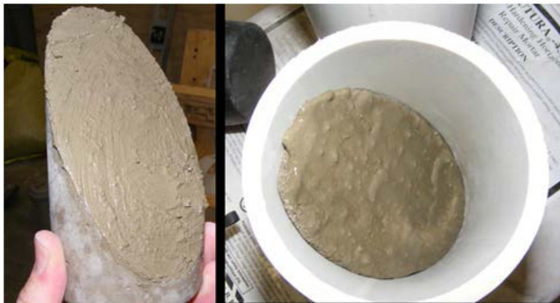
Figure 60: Mortar paste on the half cylinder prior to patching mix placement.
