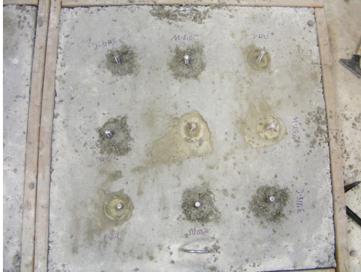
Figure 3-9 Pullout slab filled with core pullout specimens
