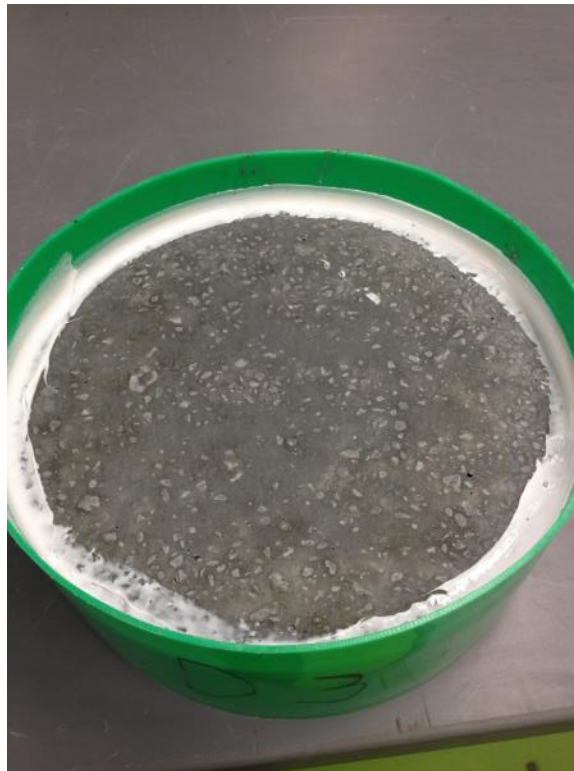
Figure 12: Scaling resistance to deicing chemicals specimen.
