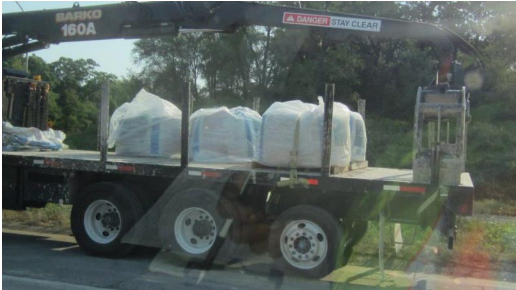
Figure 83: Truck loaded with the pre-bagged rapid set cementitious material
