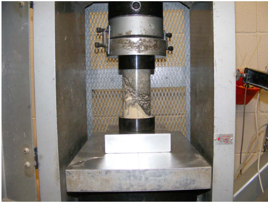
Figure 3-8 Slant shear specimen in Forney compression testing machine
