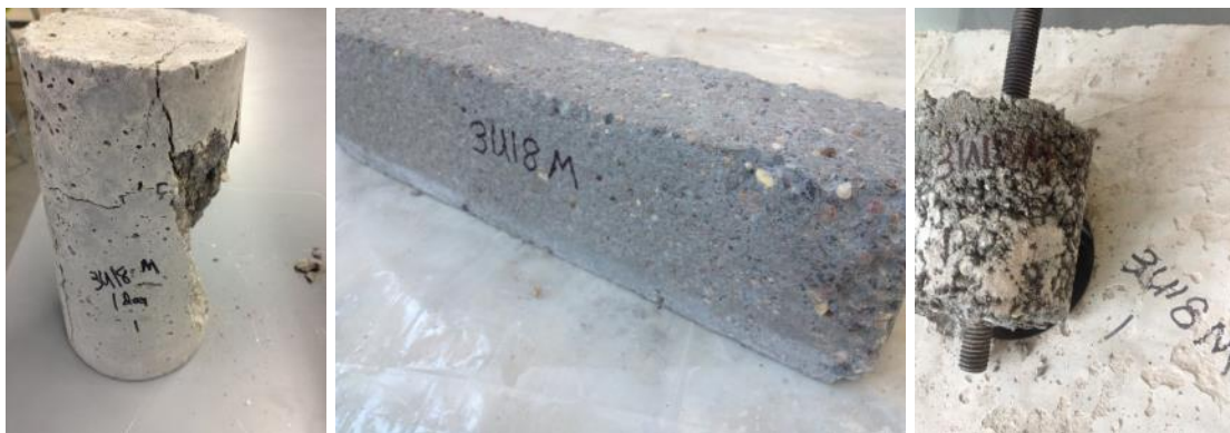
Figure 36: 3U18M compressive, freeze-thaw and pull out specimens
