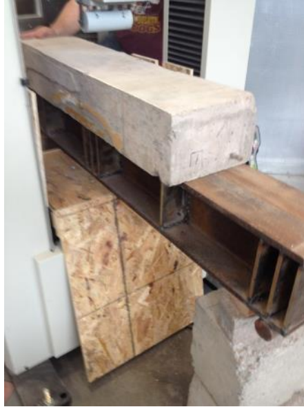
Figure 22: Half slab in the MTS loading frame
