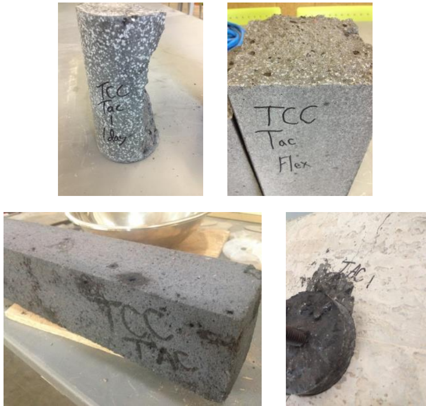
Figure 48: TCC taconite mix compressive, freeze-thaw, flexural and pull out specimens
