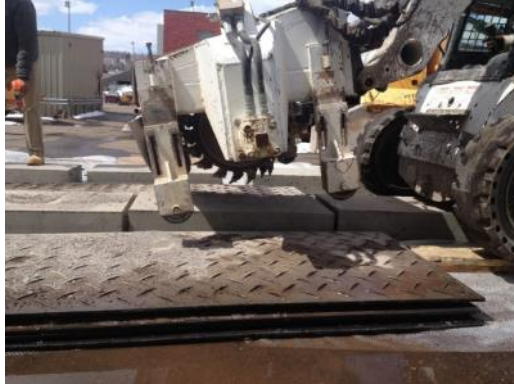
Figure 17: Pavement milling machine used to groove test slabs.
