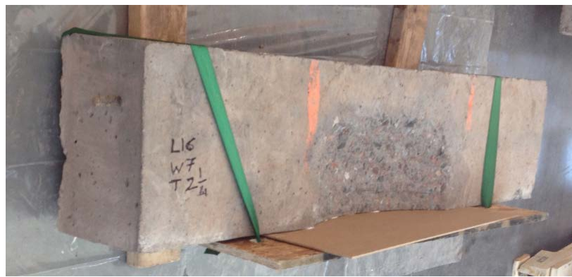
Figure 20: Half slab ready to have patching material added.
