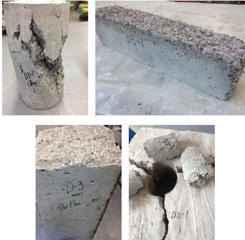
Figure 38: District 3 Mix 1 compressive, freeze-thaw, flexural and pull out specimens
