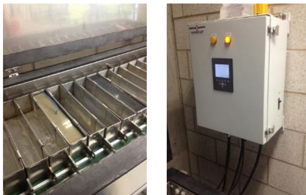
Figure 5: Freeze-thaw chamber and digital control box
