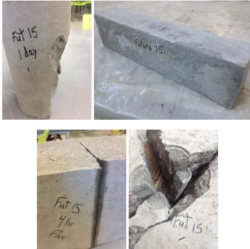
Figure 41: Futura-15 compressive, freeze-thaw, flexural and pull out specimens
