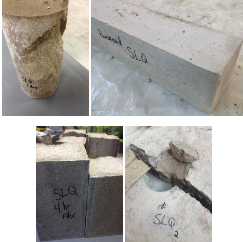
Figure 45: Pavement SLQ compressive, freeze-thaw, flexural and pull out specimens
