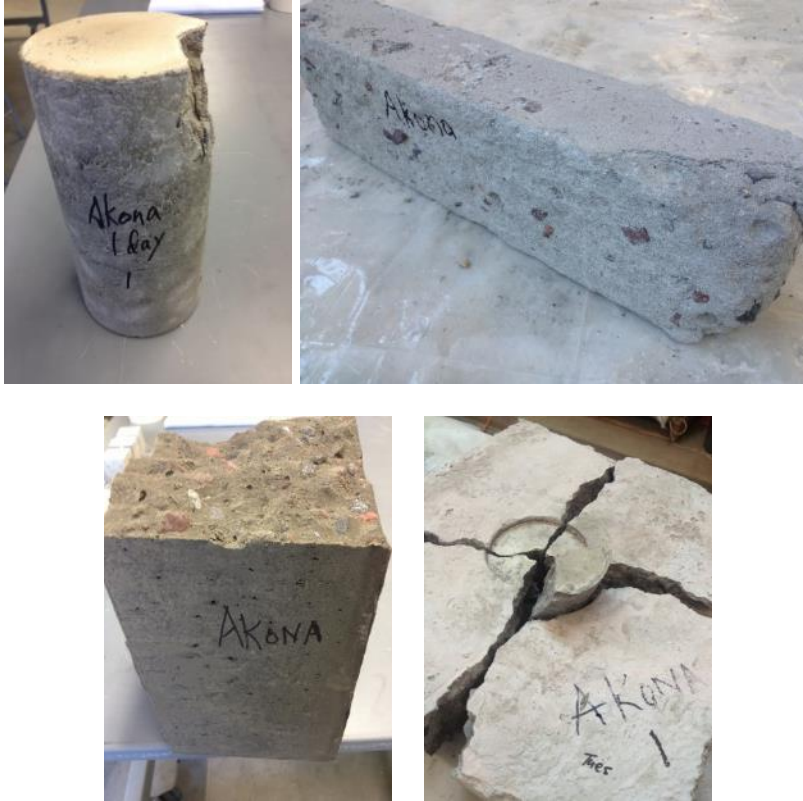
Figure 37: Akona compressive, freeze-thaw, flexural and pull out specimens
