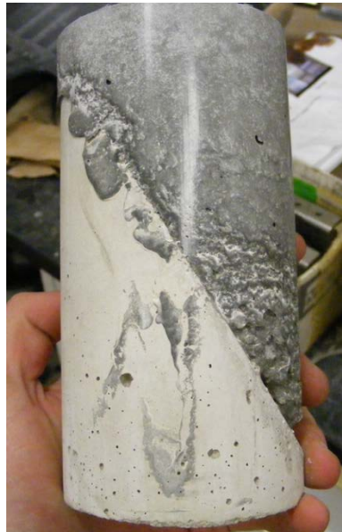
Figure 3-7 Mortar and 3U18 composite slant shear cylinder
