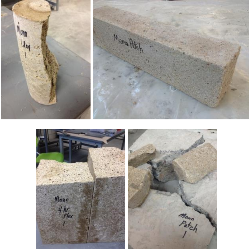
Figure 43: Mono Patch compressive, freeze-thaw, flexural and pull out specimens
