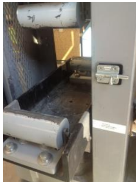
Figure 3: Third-point Bending Test Fixture in Compression Frame
