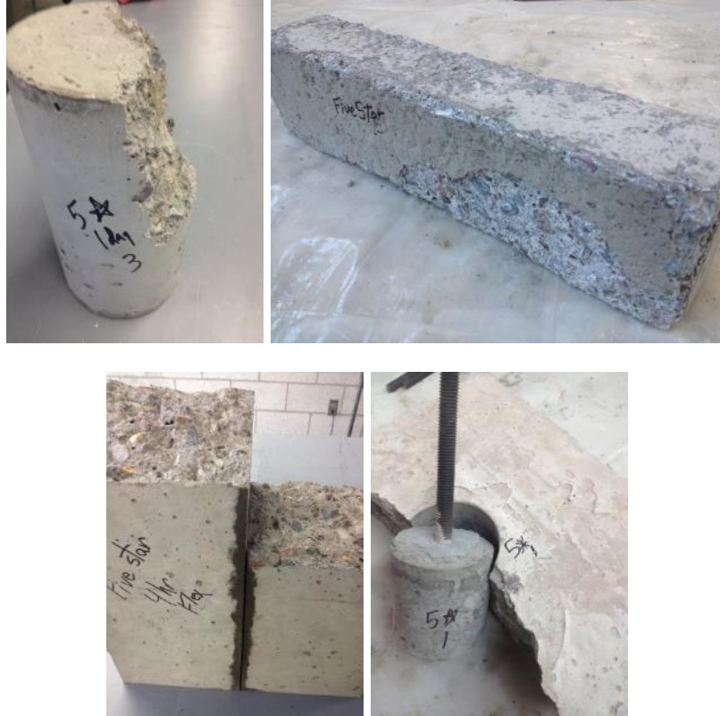
Figure 40: Five Star compressive, freeze-thaw, flexural and pull out specimens
