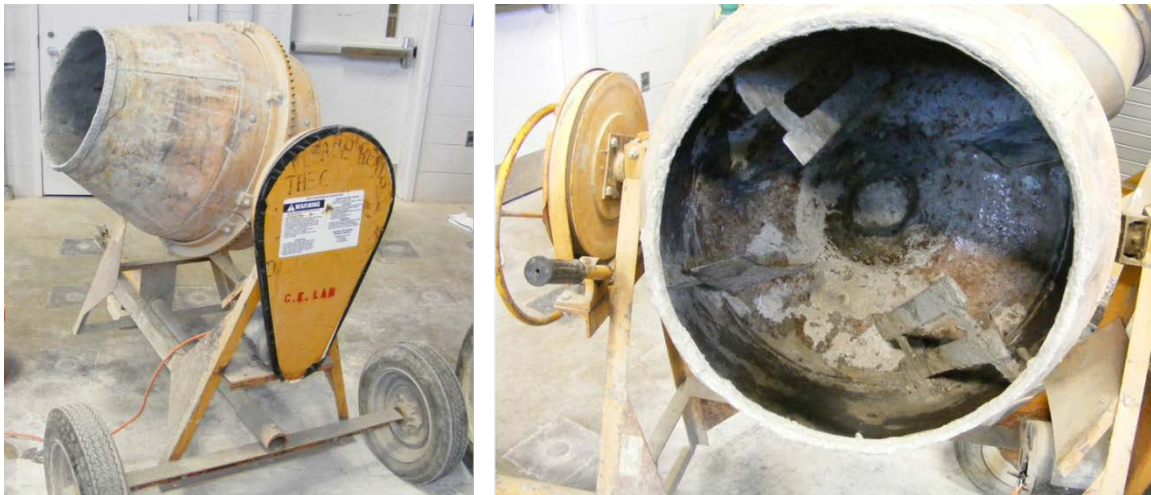
Figure 3-1 Mortar mixer used for mixing patching materials
