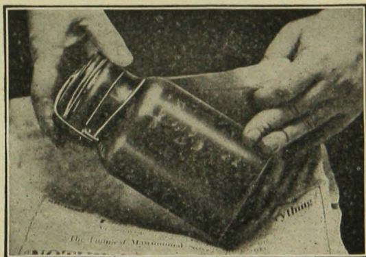
Fig. 5. Testing Finished Product The wire lever has been pressed down.
