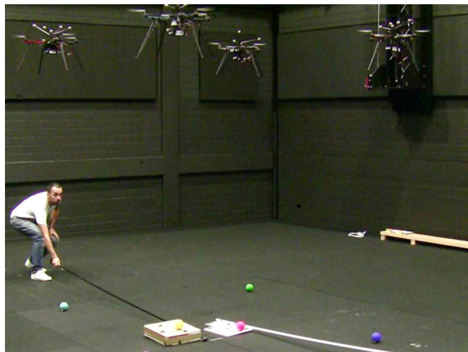
Figure 5.6: Experimental setup. Each robot is fitted with a downward facing wireless camera. All robots directly communicate with a central computer.
