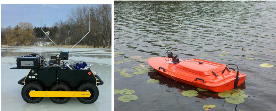
Figure 7.2: Robotic sensing system for monitoring radio-tagged carp in lakes. A directional radio antenna is mounted on a pan-tilt unit. In winter, the system employs a wheeled robot to operate on frozen lakes.
