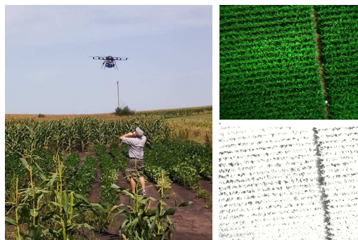
Figure 6.8: Preliminary field experiment with a UAV carrying a multi-spectral camera in a corn plot in Janesville, MN, U.S.A. Visible and near-infrared images shown were obtained from an altitude of 30 m during the experiment.
