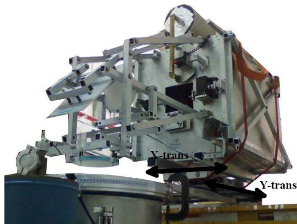
Figure 5.3: EF device with X/Y-translation stage used for receiver-only calibration measurements.
