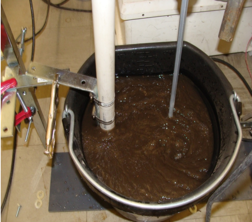
Figure 2.5. Measuring turbidity with test apparatus
