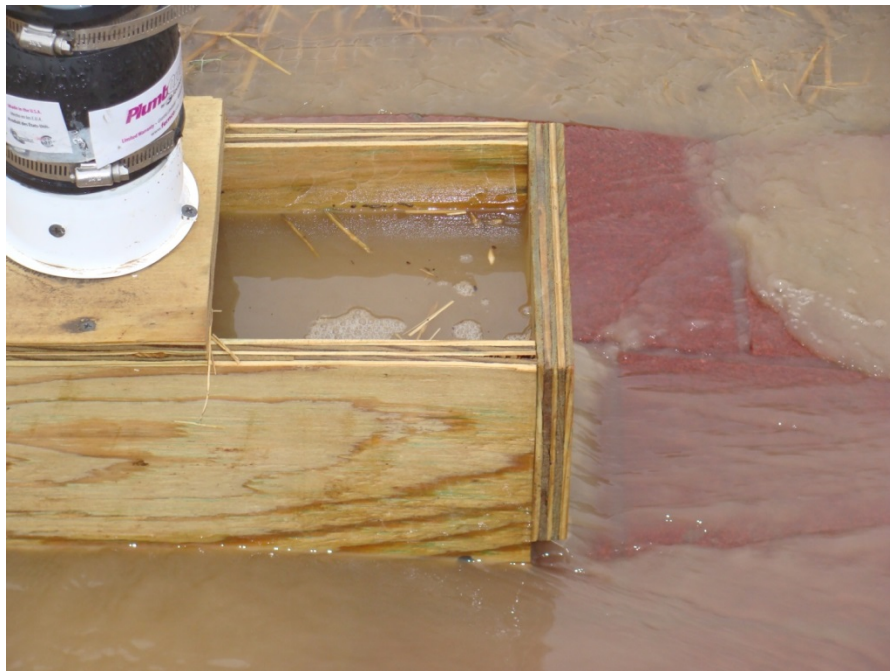
Figure 5.8. Operation of bed load slot under low flow conditions
