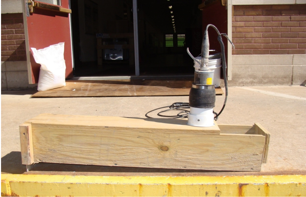
Figure 5.1. Turbidity box showing size, probe placement and overflow outlet.
