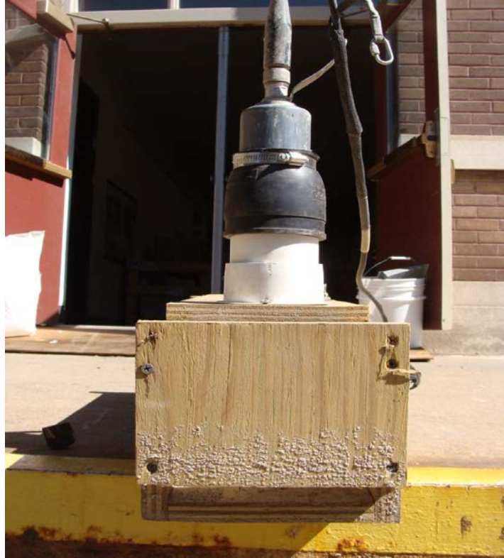
Figure 5.3. Downstream end with 0.5 inch slot opening for bed load passage
