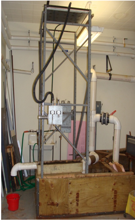
Figure 2.2. Rainfall simulator used for the laboratory experiments.
