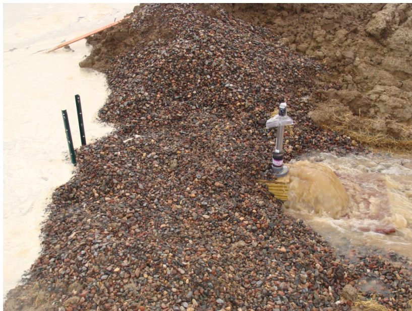
Figure 5.25. Turbidity box in rock filter with Analite 495 probe
