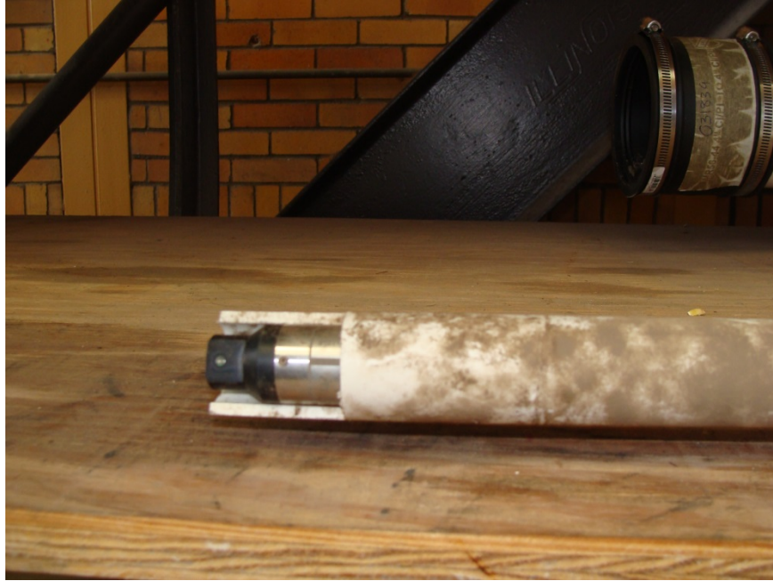
Figure 5.14. Turbidity probe mounted inside 2.5 centimeter PVC pipe for protection
