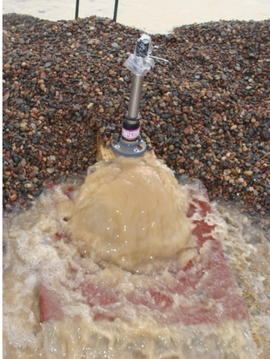
Figure 5.7. Discharge out the top of the box maintains sediment in suspension
