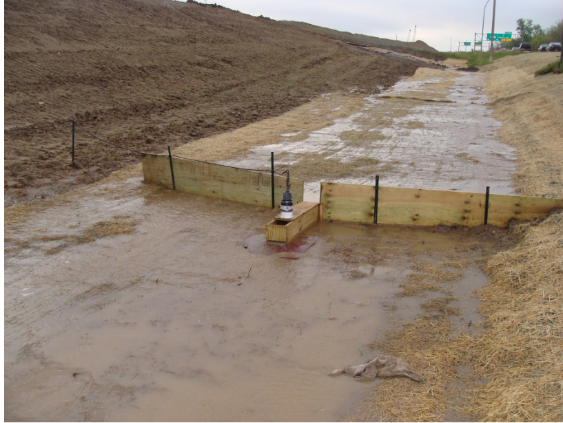
Figure 5.26. Turbidity box in ditch at Snelling/694 site just above outfall off the construction site
