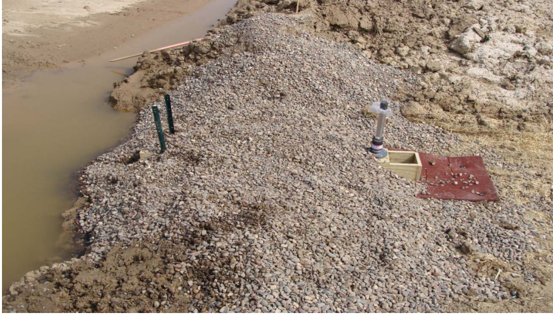
Figure 5.4. Turbidity box mounted in rock filter. Rubber mat anchored at downstream end to reduce scouring.
