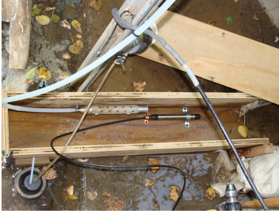
Figure 5.9. Pressure transducer, automated water sampling tube and single sample siphon bottle installed in turbidity box
